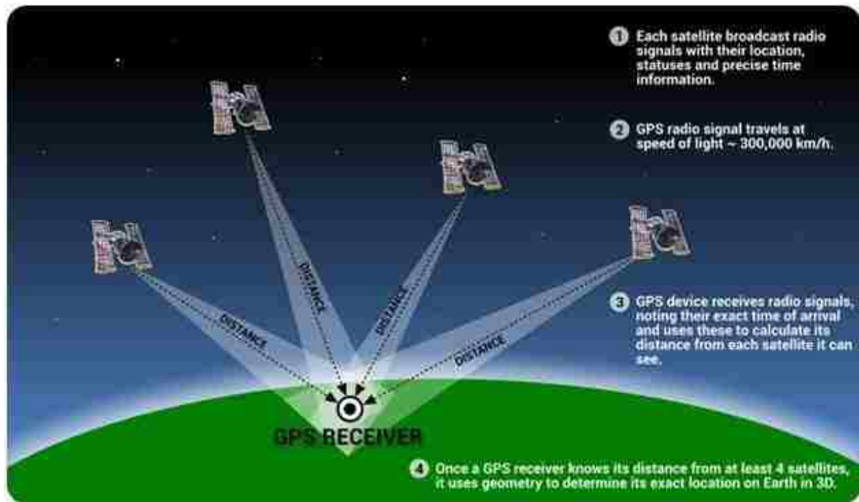
Figure 2-8 How GPS works [67]
