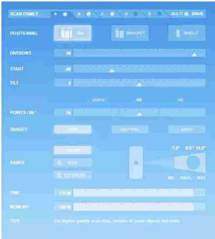
Figure 15: HMI of the laser scanner, showing list of possible settings for scanning
