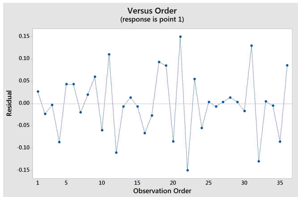
Figure C-2: Graph of the distribution of residuals vs observation order for Point 1 (forming).
