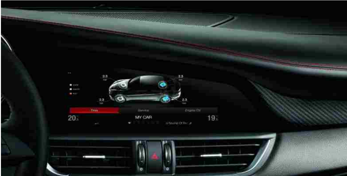
Figure 4: Integrated bezel covering the entire surface of the display [6]. (Alfa Romeo Giulia)
