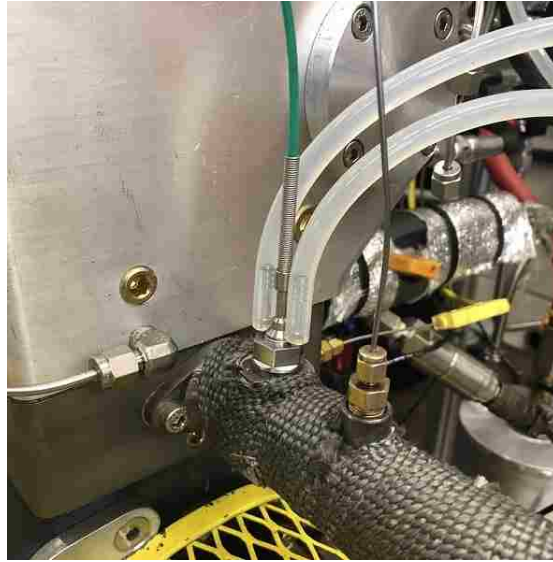
Figure 2.7: Exhaust Pressure Transducer Location
