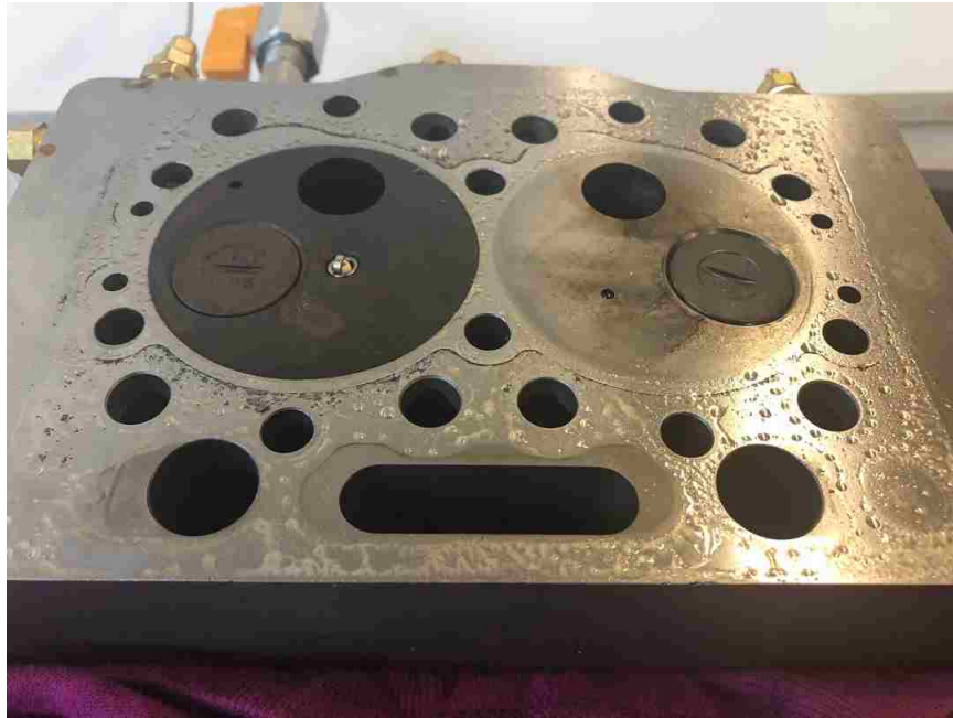
Figure 4.9: Cylinder Head exposed to Combustion Chamber
