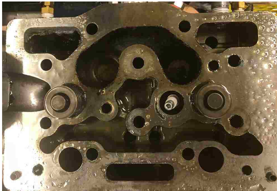
Figure 4.8: Lower head portion after removal
