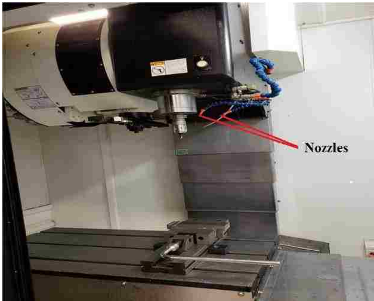
Figure 3.3 Coolant supplied through nozzles in CNC milling machine.
