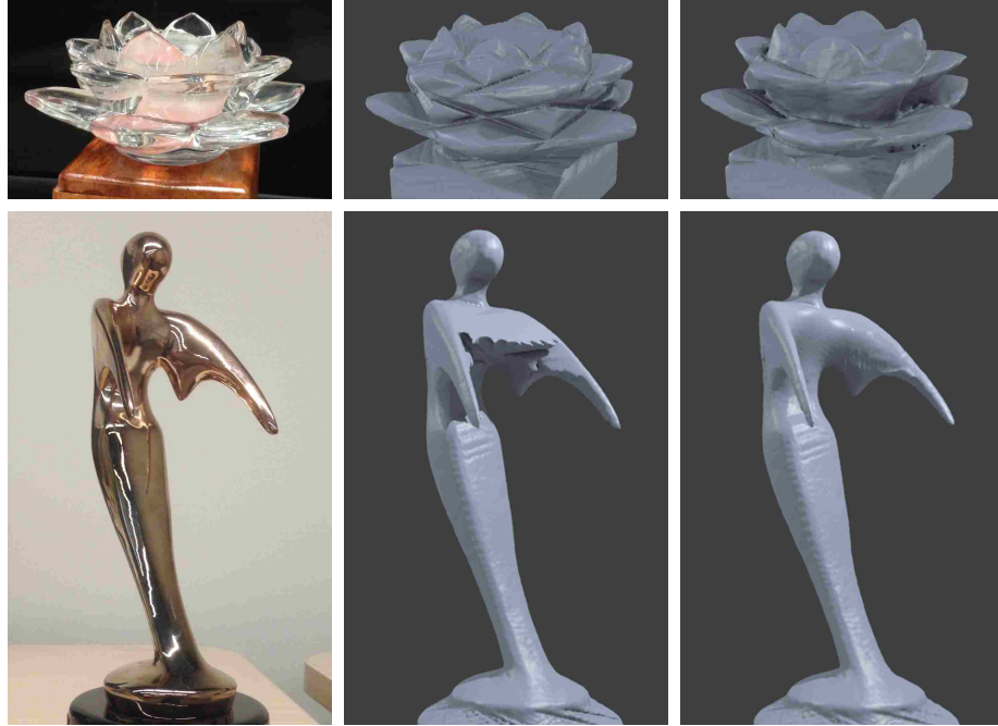
Figure 6.1: The reconstructed models for glossy trophy and glass sculpture. The left column shows the capture object; the middle column shows the reconstructed 3D model using visual hull; and the right column presents the reconstructed surface using our proposed method.
