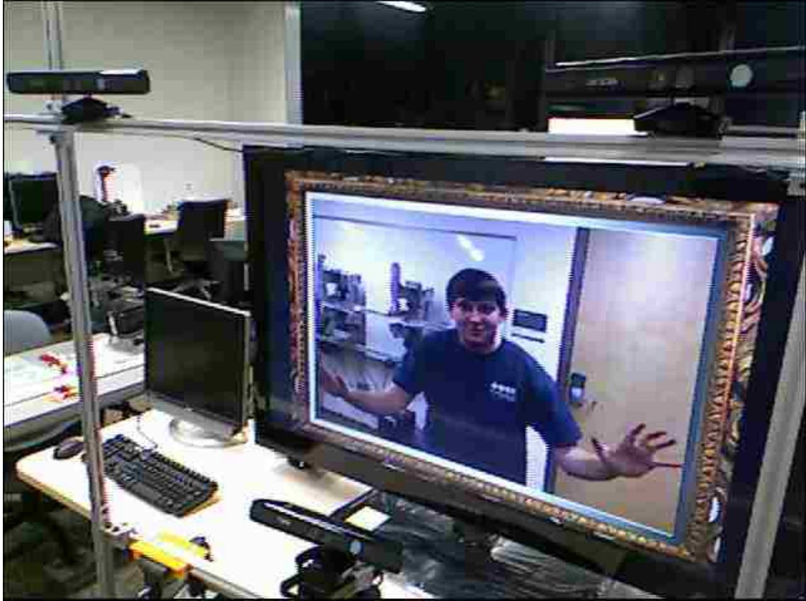
Figure 1.3: System Setting: three Kinects are mounted around the display for 3D data capturing.
