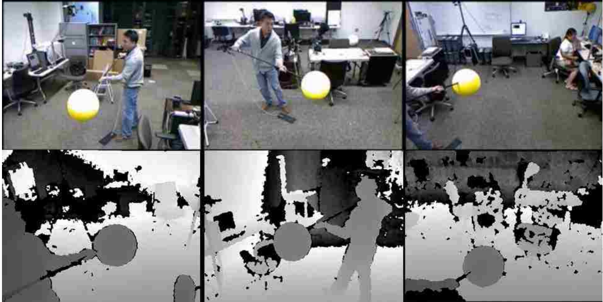
Figure 5.1: System setting for calibrating multiple color and depth camera network: the first row shows captured images from color cameras; the second row shows the ones from depth cameras.
