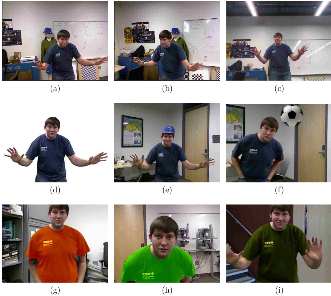
Figure 4.22: Mirror View Results II: the first row shows the original input frames from three Kinects: (a) left view, (b) right view, and (c) bottom view; (d) is the synthesized foreground view from the subject's viewpoint. (e)-(i) demonstrate different virtual mirror views by using different 3D background and inserting novel 3D objects.
