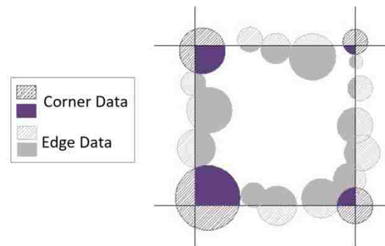
Figure 4.2. A schematic of a tile with the two types of boundary data. The solid-colored tree crown pieces inside the tile should be unified with the corresponding stripe-colored parts outside.
