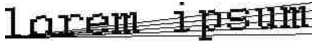
Figure 2.9: The Hough transform projects lines through pixels and counts the intersections to find the mean line and the baseline.
