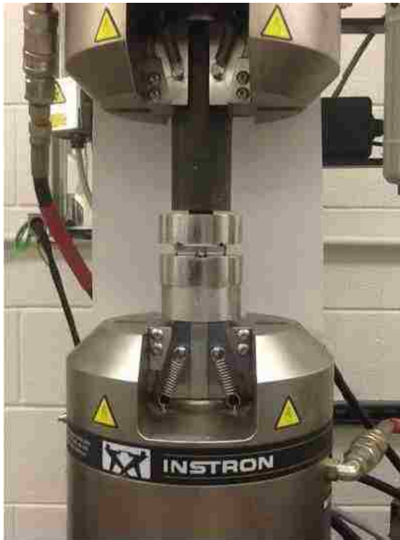
Figure 2.2 Instron-8802 testing machine for four-point bend fatigue tests.
