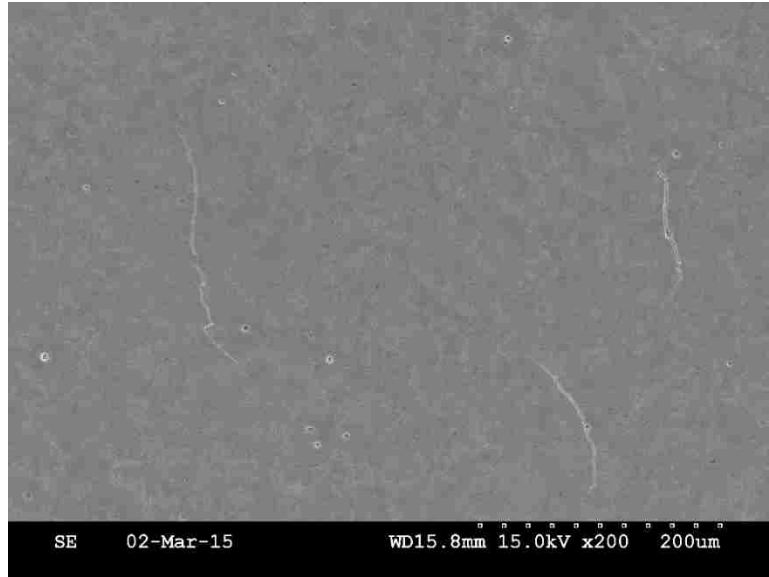
Figure 6.7 Surface cracks initiated from pores at stress level of 110% \sigma_y in alloy B.
