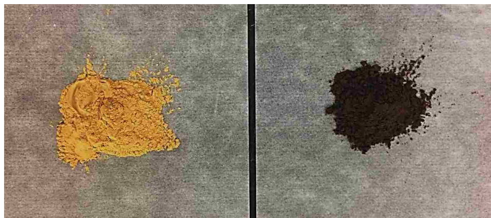
Figure S4.6 Powders crushed from (a) Fe-doped LZO pellets sintered in Ar, and (b) Fe-doped LZO pellets sintered in \text{O}_2 .
