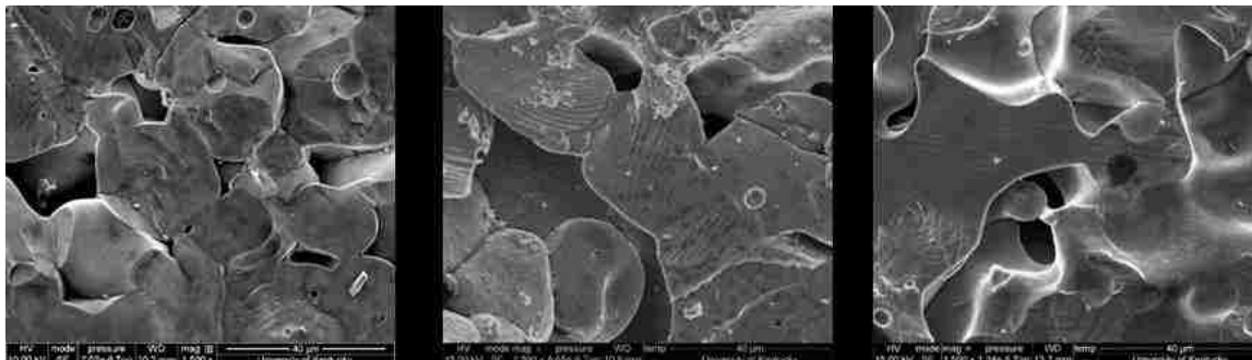
Figure S3.1 SEM micrographs of the fracture surface of sintered pellets. From left to right: 10LLZO, 15LLZO, and 20LLZO pellet.
