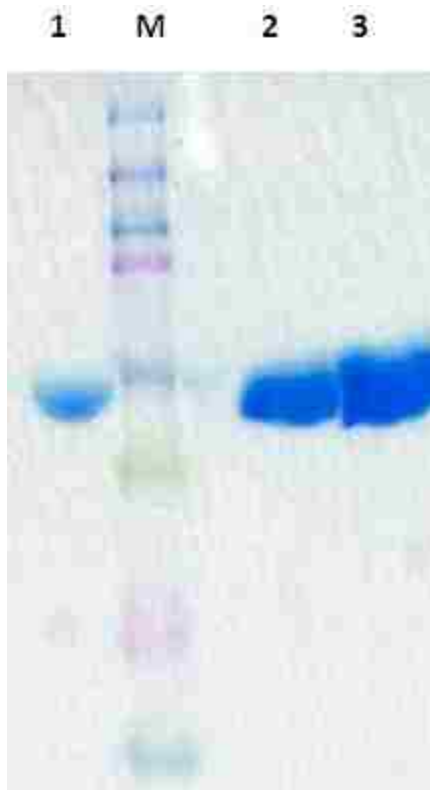
Figure 4.15 Representative SDS-PAGE of OleD Loki released from AAO membrane after one-step capture process. Lanes: 1) pure OleD Loki; M) standard molecular weight markers; 2) 7 \mu\text{g} captured OleD Loki released from AAO membrane; and 3) 14 \mu\text{g} captured OleD Loki released from AAO membrane. Lanes 2 and 3 were purposefully overloaded to delineate potential impurities associated with the capture method.
