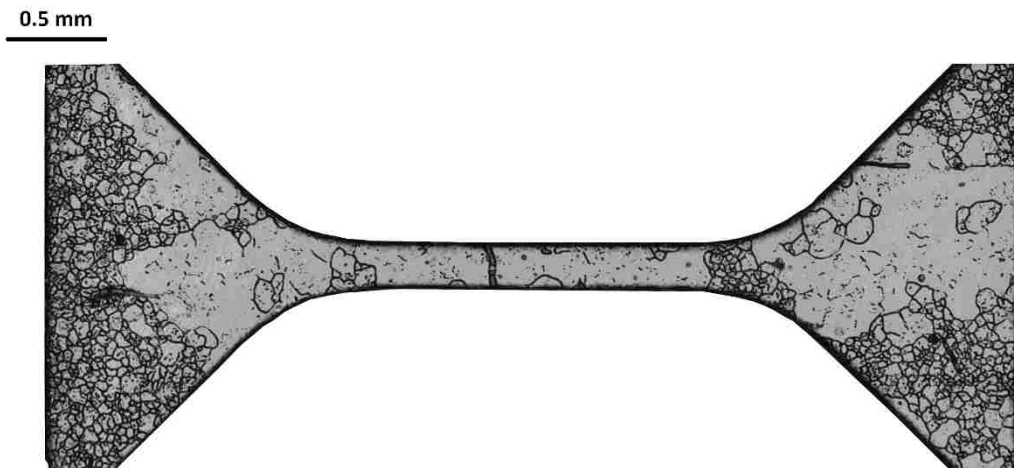
Figure 5.4. Optical micrograph of a tensile testing specimen with dogbone shape, after extraction by wire EDM. Some grain boundaries can be seen to still be present in the gage section, despite the grain size reached by AGG.
