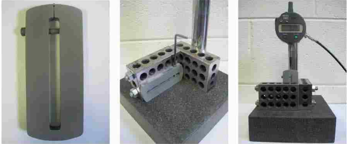
Figure 8.1. (left) custom made specimen holder used to clamp the specimen in proper position to ensure perpendicularity of the ends with the long axis, (middle) holder in position against angle plate and granite stand to position the specimen and (right) verification of the final polished end face using a comparator. (images reproduced from Michael Bürckert Master thesis)
