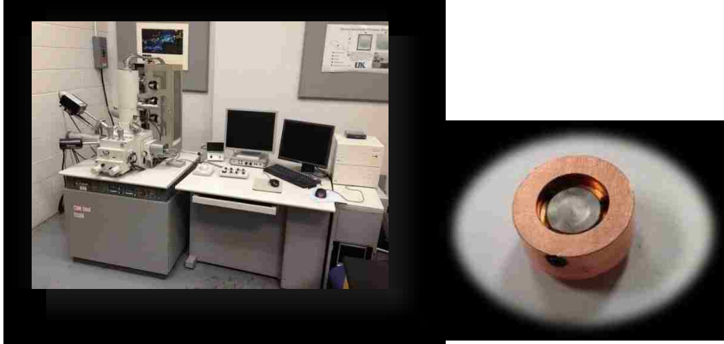
Figure 3-8. Hitachi S4300 scanning electron microscope and custom copper sample holder for machined porous tungsten samples. The holder substantially improved image quality by draining electrical charge efficiently.
