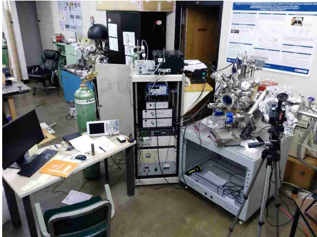
Figure 3.9 The cathode characterization chamber and associated electronics.
