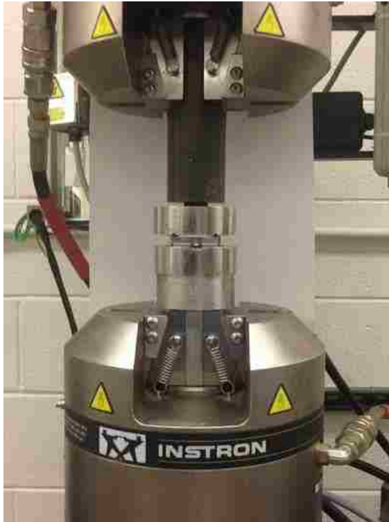
Figure 2.3 The actual four-point bend fatigue test rig during fatigue testing.
