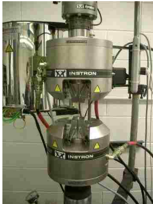
Figure 2.2 The Instron 8800 servo-hydraulic test machine used for the tensile testing.
