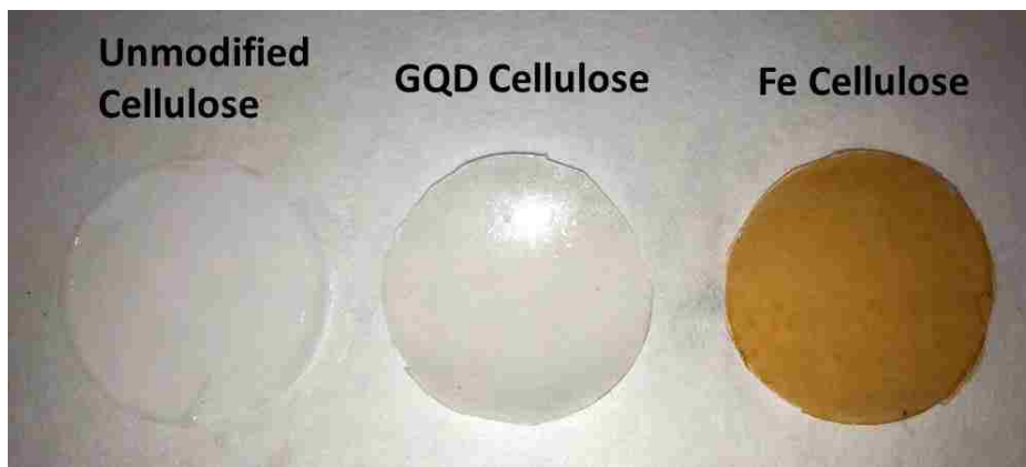
Figure 6.1. Unmodified cellulose, GQD cellulose, and iron cellulose composite membranes.
