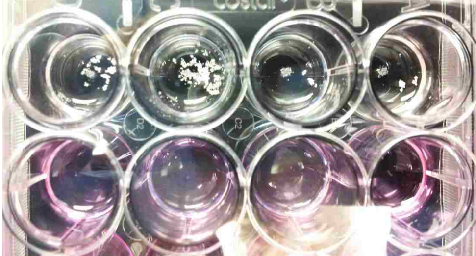
Figure 68: Particles in wells after adding the supernatant. As an example the undiluted and 1 st dilution wells of the 1 week supernatant of the alloy sample is shown. From the 2 nd dilution on, no particles were observable by naked eye.
