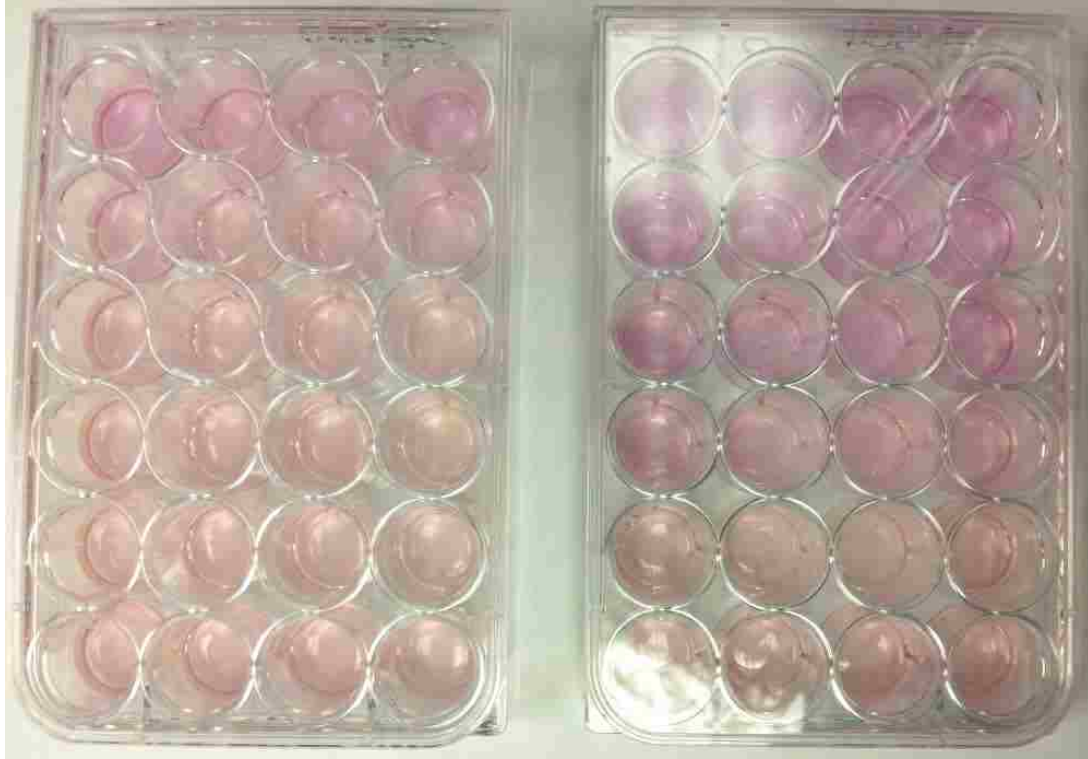
Figure 71: Milled magnesium supernatants after 24 h exposure to cells. On the left the supernatant prepared for 24 h and on the right the 1 week supernatant.
