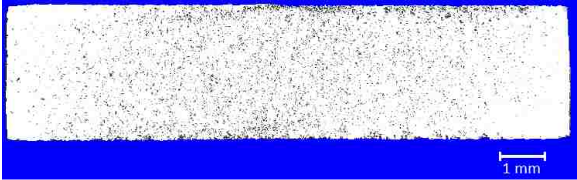
Figure 29: Cut through Mg_{65}-Ti_{35} sample sintered in WC die.
