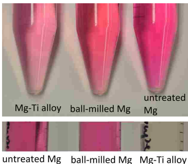
Figure 63: Supernatant color after incubating the samples for 24 h (left) and 1 week (right).
