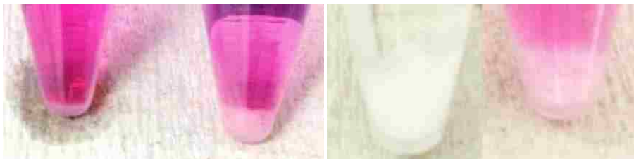
Figure 67: On the far left is the unmilled magnesium supernatant prepared for 24 h. No white crystals can be seen at the bottom of the centrifuge tube, which is representative for all 24 h supernatant solutions. To its right is the 1 week unmilled magnesium supernatant, in which white crystals have accumulated at the tip of the centrifuge tube. The right image shows the crystals in the alloy supernatant (left) and milled magnesium supernatant (right), both incubated for 1 week.
