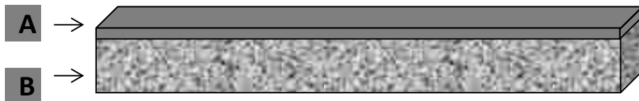
Figure 1.2: Schematic representation of an asymmetric flat sheet membrane. (A) \sim 0.1\text{-}1\ \mu\text{m} thick dense layer, where gas separation occurs via solution diffusion (B) \sim 100\text{-}200\ \mu\text{m} thick porous layer, which provides mechanical support.
