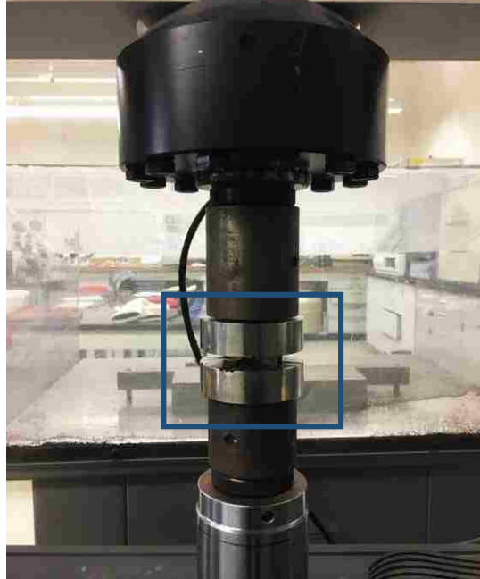
Figure 2.4 MTS 810 servohydraulic material testing system, the square shows the four-point bend fatigue testing rig.
