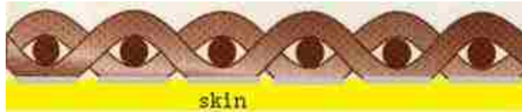
Figure 2.16 Side view of polished wire mesh in contact with skin. In unpolished areas aluminum is insulated by PAC coating so electric discharge is confined to the bottom plane. The silver segments show exposed aluminum acting as electrodes for electroporation.
