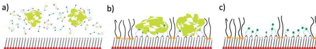
Figure 6.1. Schematic representation of our proposed approach towards molecularly imprinted monolayers using thiol-yne click chemistry. A) Monolayer is exposed to a mixture of ligands and template protein. Ligands bind to template proteins as well as thiolated surface. B) UV irradiation locks ligands onto surface. Unreacted regions on thiolated surface are backfilled with PEG-maleimide. C) Surface is rinsed with surfactant to release the template proteins.
