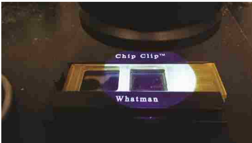
Figure A-1.2: Photograph of the UV photodegradation apparatus. Collimated LED outputting 365 nm light with a ChipClip / FAST-slide assembly.
