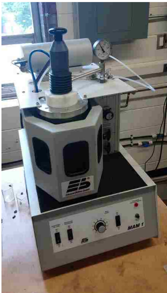
Figure 3.3. Mini arc-melting (MAM) system by Imteck, available at Dr Balk's research group at the University of Kentucky
