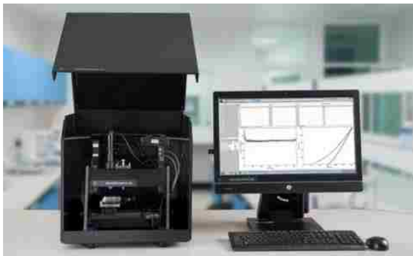
Figure 3.10. iNano nanoindentation instrument 10
