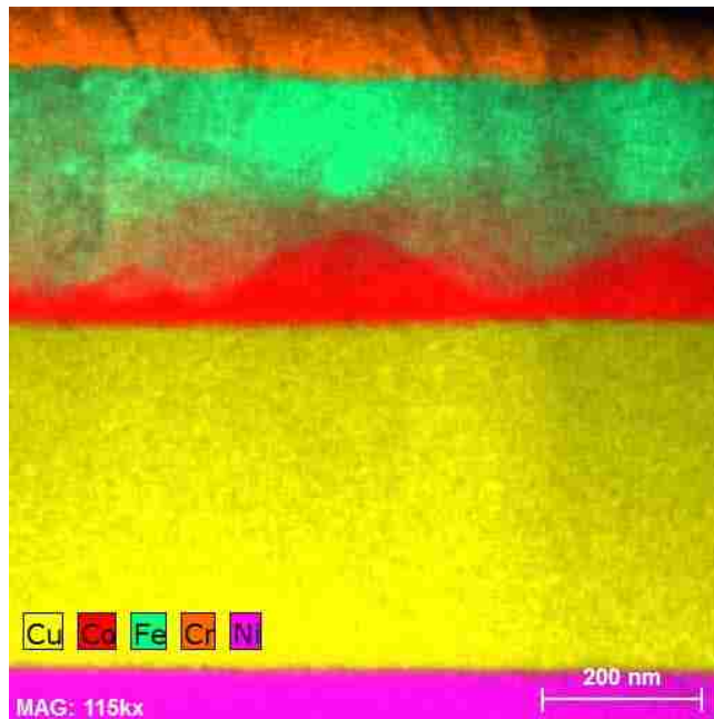
Figure 7.4. Electron image and the EDS map collected from the alloyed sample by the Talos TEM
