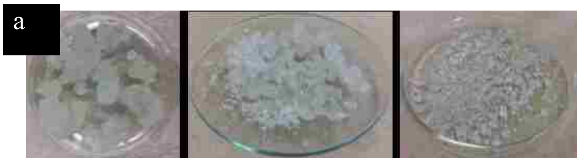
Figure 4.3: Drying crushed polymerized GMA product over a week
