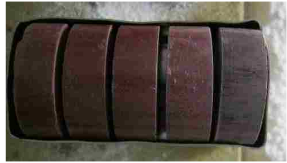
Figure 3-5: Top view of the arrangement of the pellets in the platinum crucible
