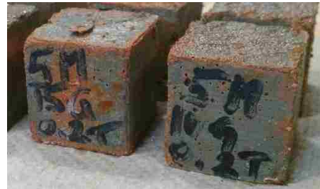
Figure 6-13: Mortar cubes of clinker#5-MBP+10/15G+0.2T after 28 days of hydration
