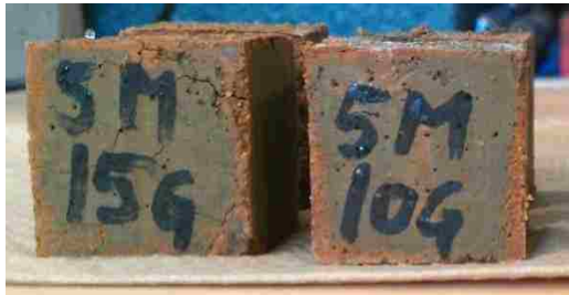
Figure 6-12: Mortar cubes of clinker#5-MBP+10/15G after 28 days of hydration
