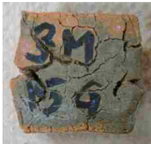
Figure 6-9: Mini mortar cube of clinker#3-MBP+15G after 28 days of hydration
