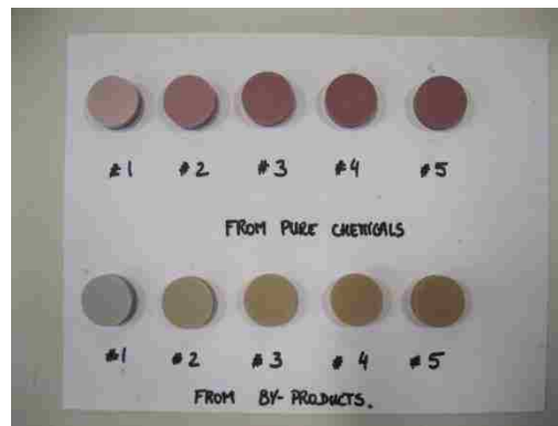
Figure 3-3: Small pellets for each batch produced from RC and BP before firing
