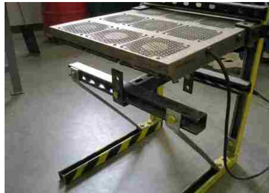
Figure 3-9: Ventilator used to quench the pellets
