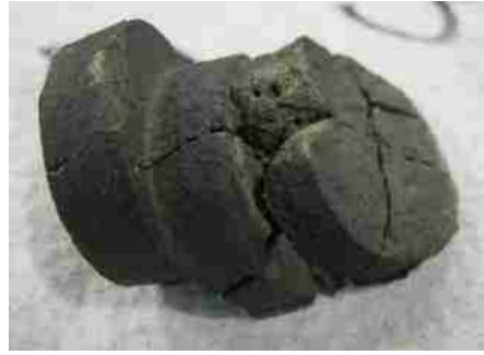
Figure 4-9: Pellets made from industrial by-products (BP) just after firing at 1300°C and quenching step
