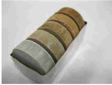
Figure 4-8: Pellets made from industrial by-products (BP) just before firing process
