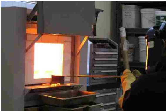
Figure 3-8: Carbolite ® furnace with front opening to facilitate quenching step
