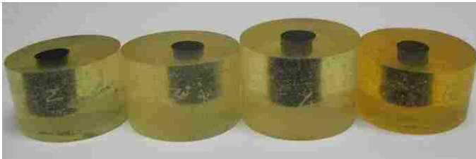
Figure 3-10: Front view of prepared epoxy samples
