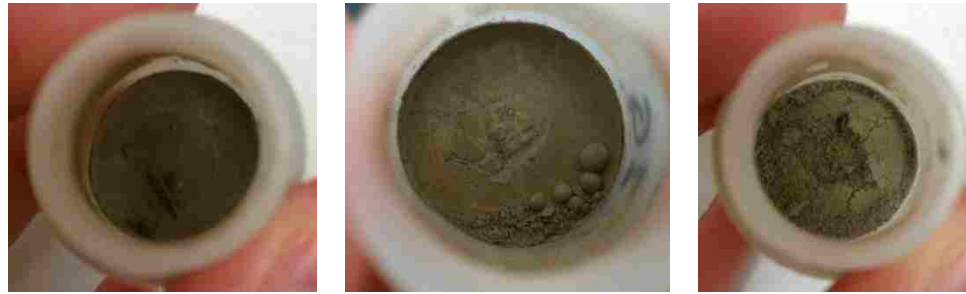
Figure 5-7: Images of several cement pastes from the inside of plastic vials, following the end of the calorimetric tests. Left image: B#3-RC+15G defined as hard cement paste (H); middle image: B#5-RC+25G defined as moderately hard/soft cement paste (H/S) and easily “scratchable”; right image: B#3-RC+50G defined as completely expanded cement paste (Ex), turned into powder-like aspect
