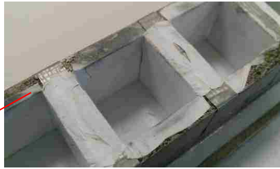
Figure 3-26: Close-up of one 1-in hollow mortar cube mold
