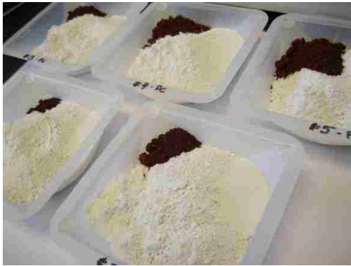
Figure 3-1: Batches produced from reagent chemicals (RC)
