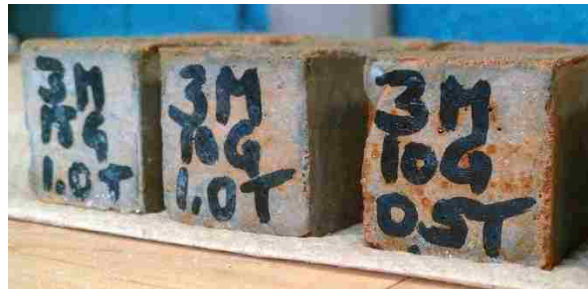
Figure 6-10: Mini mortar cubes of clinker#3-MBP+15G+1.0T, #3-MBP+10G+0.5/1.0T after 28 days of hydration
