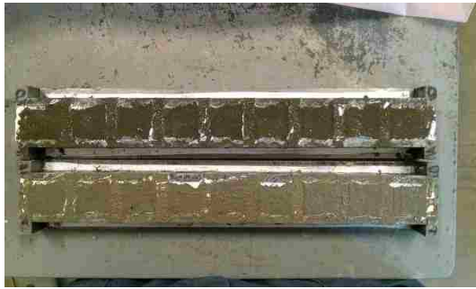
Figure 3-28: 1-in mini-mortar cube mold filled with sample
