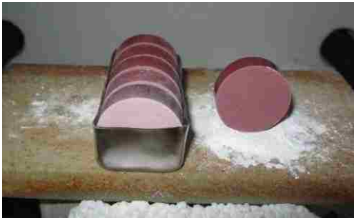
Figure 3-4: Front view of the arrangement of the pellets in the platinum crucible on the left, and on a thick layer of ZrO 2 (1-2 mm) on the right
