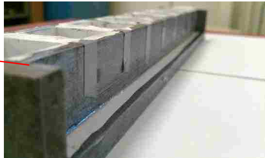
Figure 3-27: Side of the mold where petroleum is applied to prevent water leak
