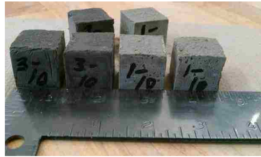
Figure 3-29: Mini-mortar cubes after demolding step
