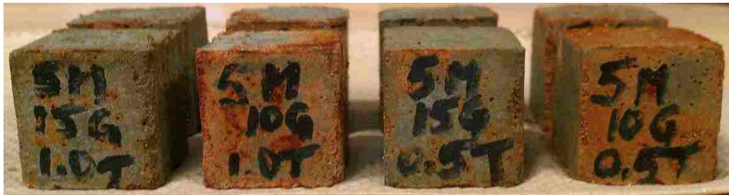
Figure 6-14: Mortar cubes of clinker-MBP#5+10/15G+0.5/1.0T after 28 days of hydration
