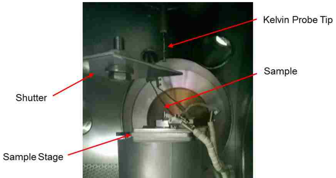
Figure 3.6 Kelvin Probe station within the UHV Chamber. Depicted are the Kelvin Probe tip, protective shutter, and the sample stage with electrical connections for resistive heating of samples.
