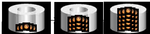
Figure 3-1: Proposed copper monolayer growth front mechanism. Copper monolayer nucleates at the conductive face of the membrane and grows through the pores of the membrane.
