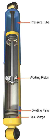
Figure 2.2: Monotube damper (figure reproduced from [3])
