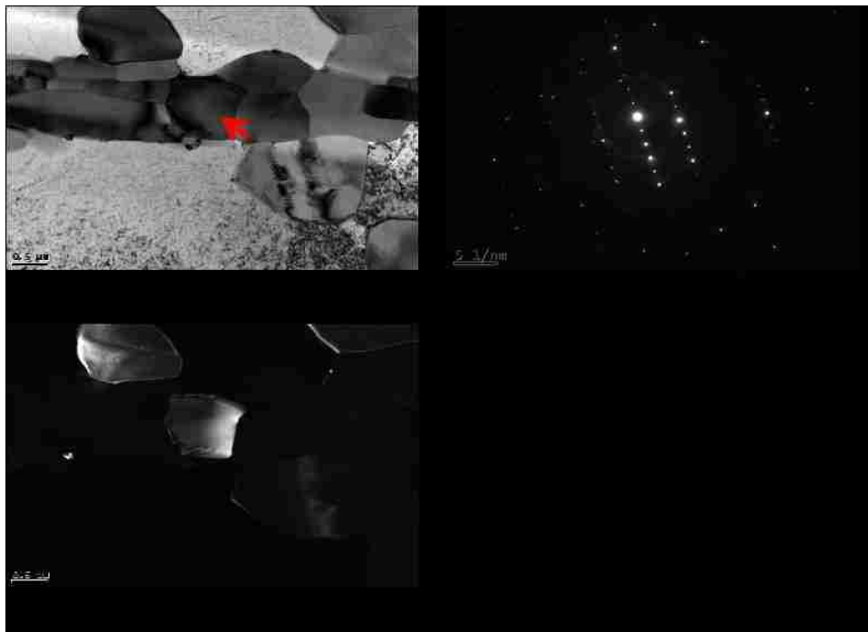
Figure 175. Bright and dark field images for the \text{Al}_7\text{Cu}_2\text{Fe} . Selected Area Diffraction Pattern (SAD), ref. # Yamaha engine block.
