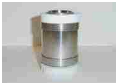
Figure 74. High Temperature UMSA test sample and TA cup assembly.
