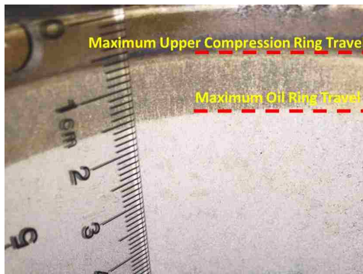
Figure 59: Dynamometer 2 - Engine 2633 - Cylinder 1 - Back – Piston Ring Travel Schematic
