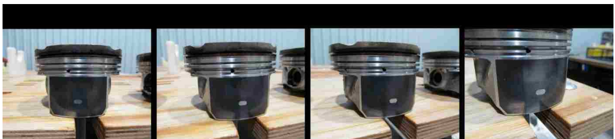
Figure 90: Dynamometer 3 - Engine 2595 - Teardown - Piston Skirts - Major Thrust Side
