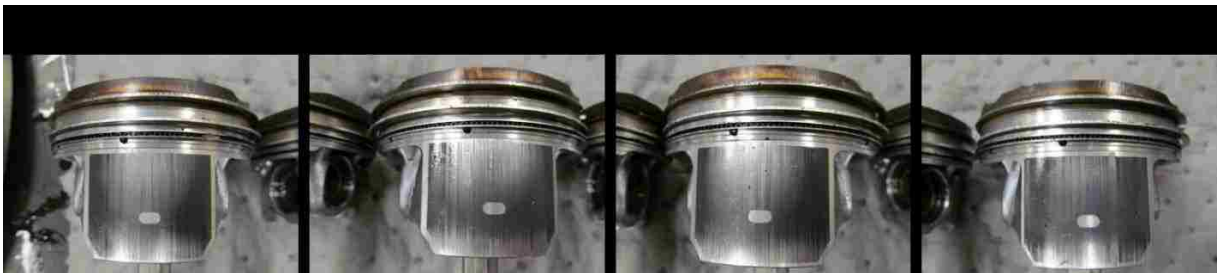
Figure 50: Dynamometer 1 - Engine 2599 – Teardown - Piston Skirts - Minor Thrust Side
