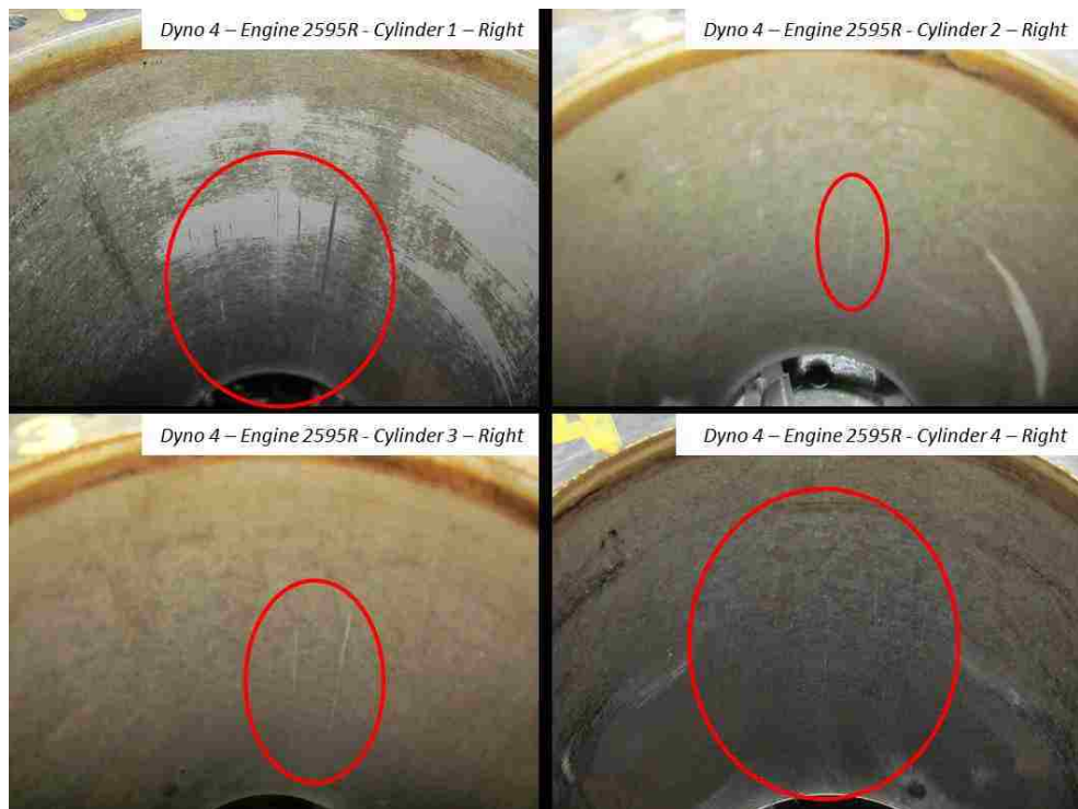
Figure 103: Dynamometer 4 - Engine 2595R - Teardown - Cylinders – Wear Marks – Major Thrust Side
