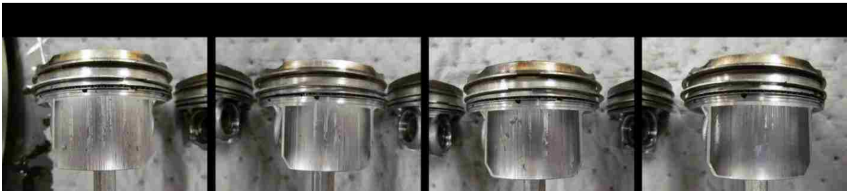
Figure 49: Dynamometer 1 - Engine 2599 – Teardown - Piston Skirts - Major Thrust Side
