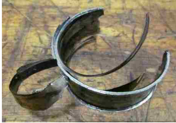
Figure 101: Dynamometer 4 - Engine 2595R - Journal Bearing - Cylinder 4
