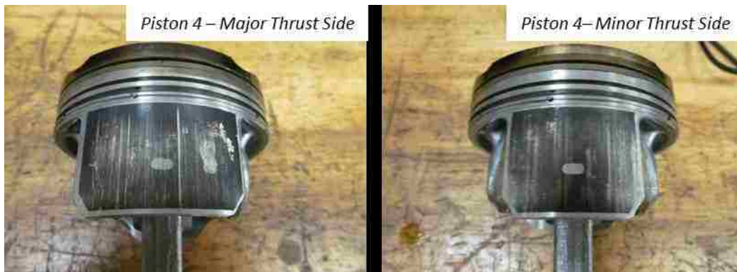
Figure 111: Dynamometer 4 - Engine 2595R - Teardown - Piston Skirts - Piston 4
