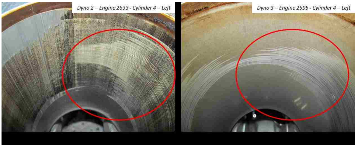
Figure 117: Discussion - Ring Flutter Wear – Comparison Between Engine Trials 2 & 3
