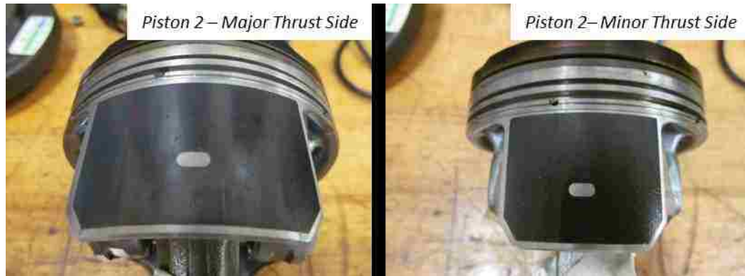
Figure 109: Dynamometer 4 - Engine 2595R - Teardown - Piston Skirts - Piston 2
