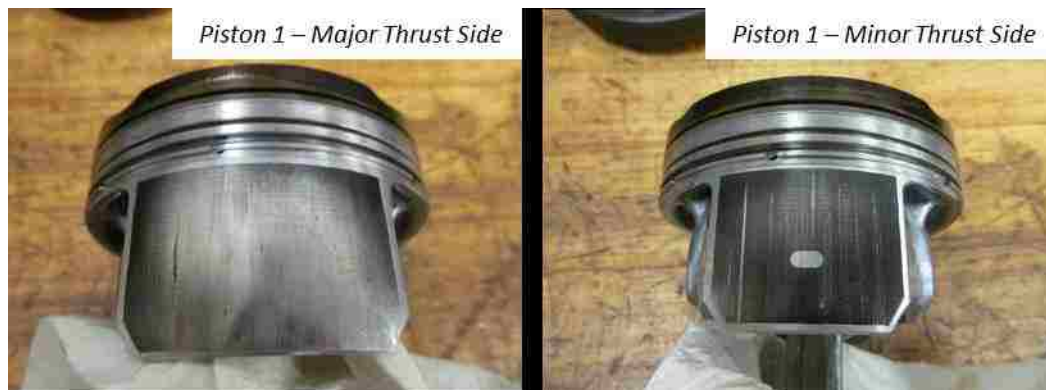
Figure 108: Dynamometer 4 - Engine 2595R - Teardown - Piston Skirts - Piston 1
