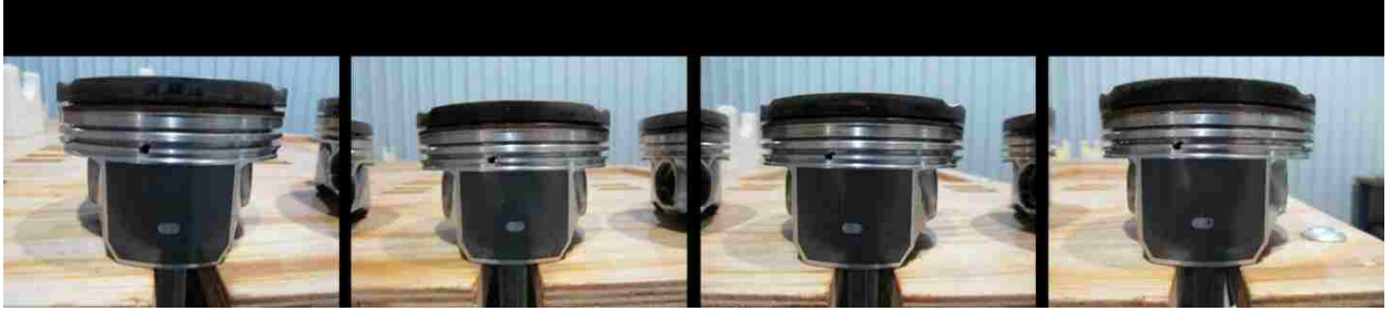
Figure 91: Dynamometer 3 - Engine 2595 - Teardown - Piston Skirts - Minor Thrust Side
