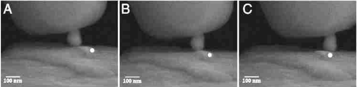
Figure 2.41: Demonstration of sliding behaviour of an IF nanoparticle. The white dot represents the initial point of sliding [93]
