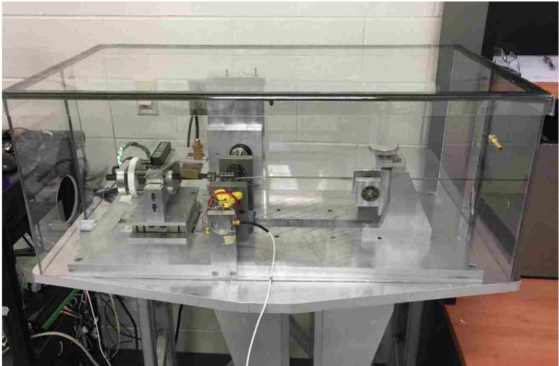
Figure 3.7 Photograph of the installation of the chamber on the tribometer.
