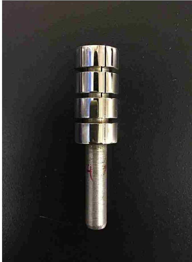
Figure 3.4 Image showing the polished pin used in the friction tests
