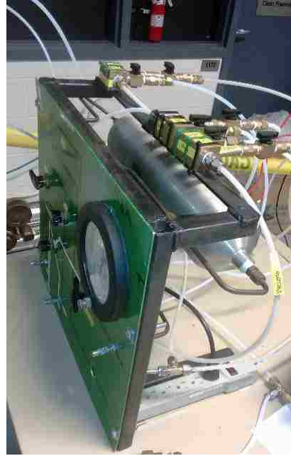
Fig. 22: The mixing chamber of the gas mixing panel
