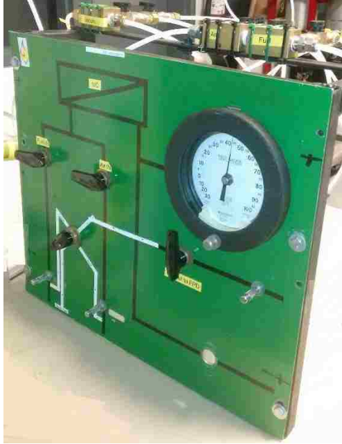
Fig. 21: Gas mixing panel front
