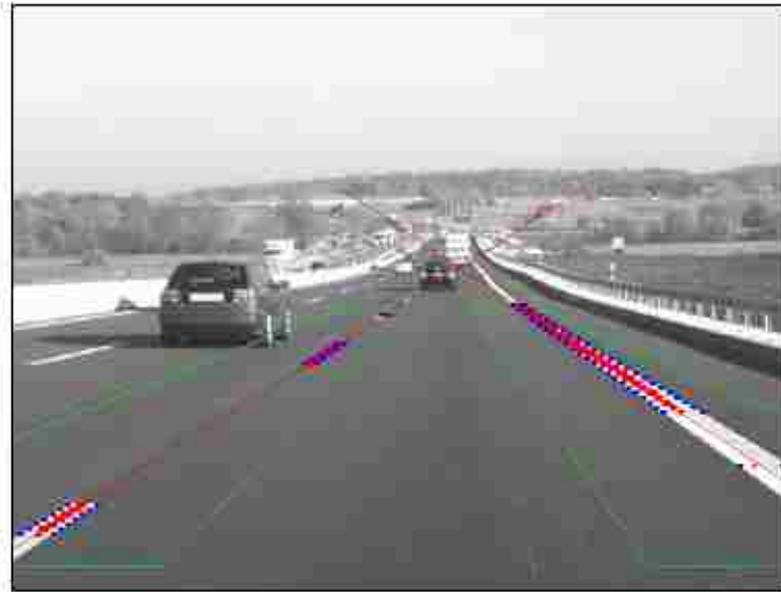
*Figure 3.6: Lane Recognition through a camera sensor*
