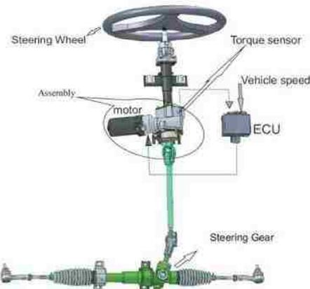
*Figure 3.9: Electric Power Steering actuator*
