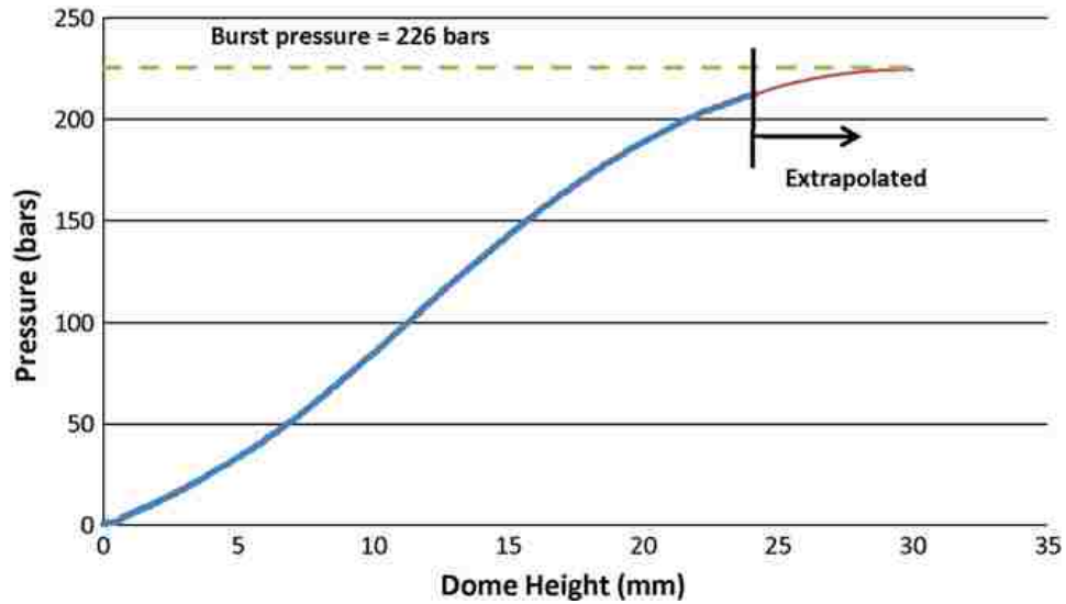
Figure 7-8. Pressure vs. dome height curve extrapolated from 212 bars to a burst pressure of 226 bars [22]
