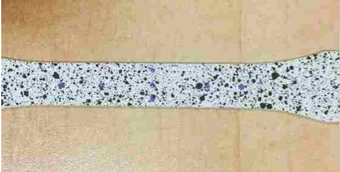
Figure 4-4. Tensile test specimen with speckle pattern
