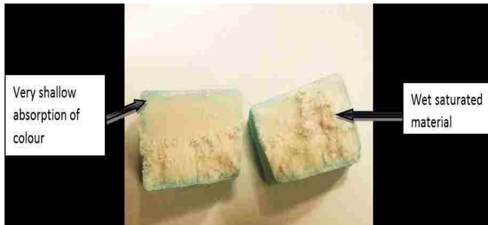
Figure 17 Epsom Salt Mixture Prepared Samples (soggy center)
