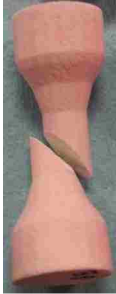
Figure 39 Compression test specimen after critical failure
