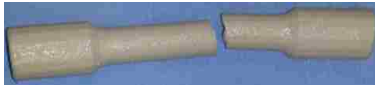
Figure 27 Tensile test specimen after critical failure
