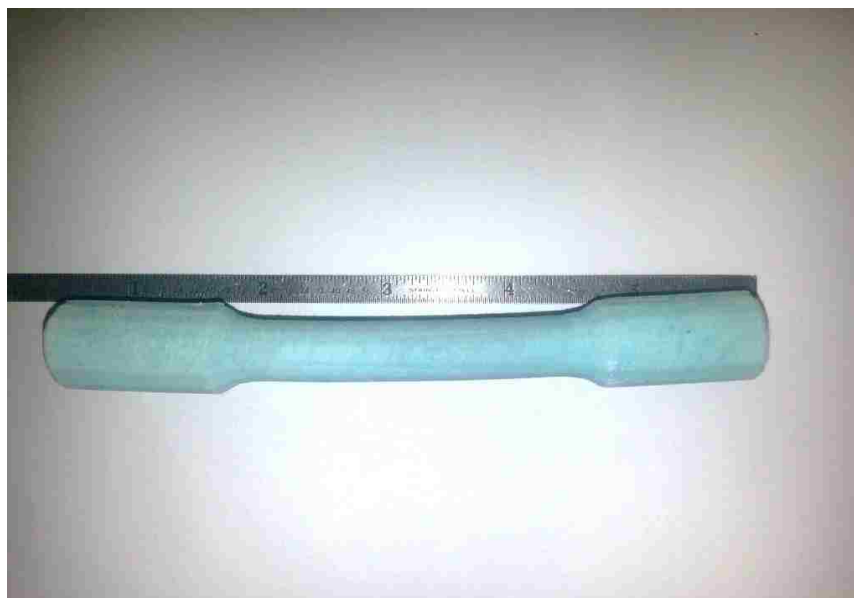
Figure 31 Deformed tensile specimen from salt mixture
