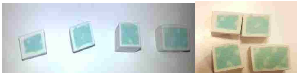
Figure 16 Diluted Cyanoacrylate w/ Non-Uniform Absorption Compared w/ Time (Low to High, L-R and CLW)
