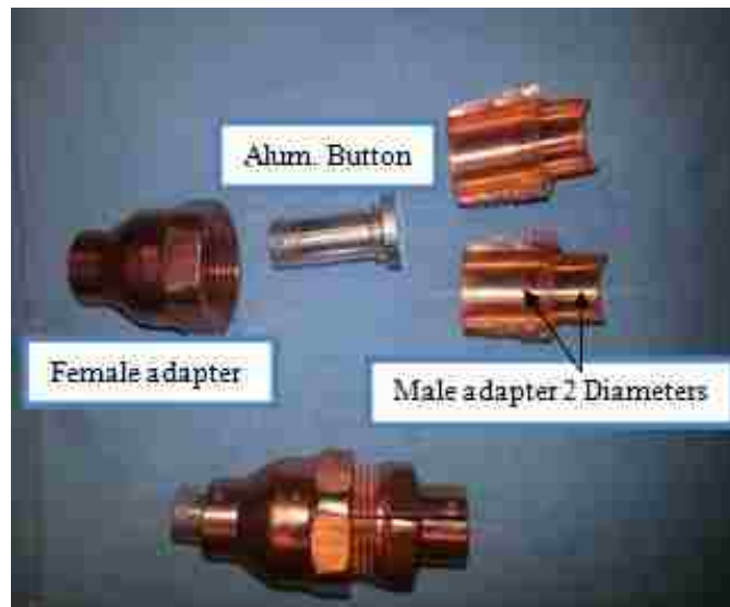
Figure 24 Parts and full assembly of tensile specimen holding fixtures
