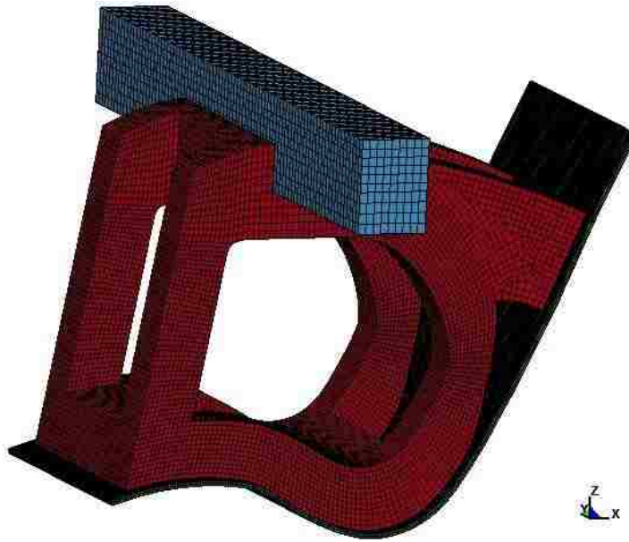
Figure 78. Modified geometry of the CRSIAD with its mesh quality.
