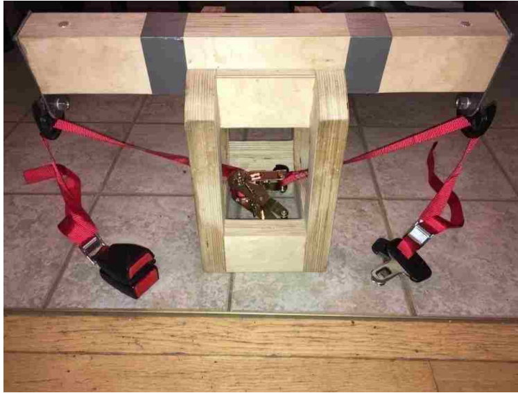
Figure 73. The complete assembly with adjustable clips installed on the ratchet webbing.
