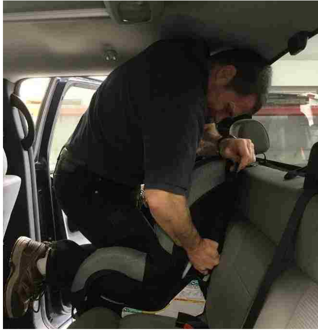
Figure 4. CRS installation for forward-facing configuration by certified CRS installer.
