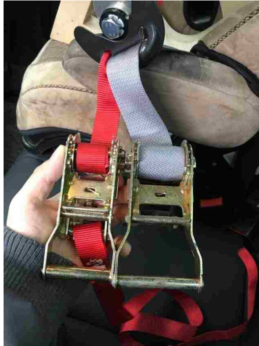
Figure 68. A comparison between the new ratchet (left) and the original ratchet (right) in terms of size and webbing.
