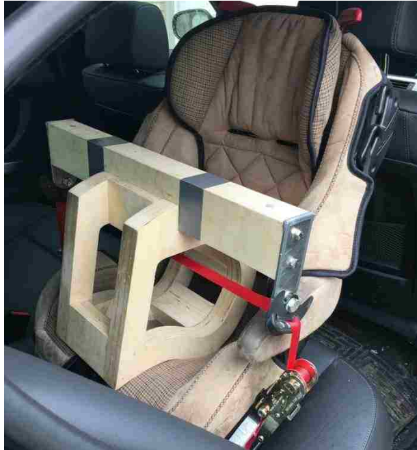
Figure 67. The Rearward-facing Configuration Preliminary Test Setup for the CRSIAD.
