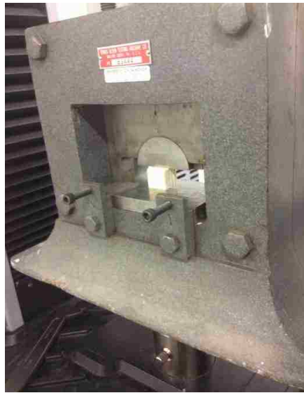
Figure 27. The setup of the specimen on the Tinius Olsen Shear Test Apparatus.
