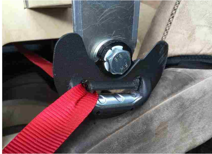
Figure 69. The downsized webbing stuck at the corner of D-ring slot while under tension.
