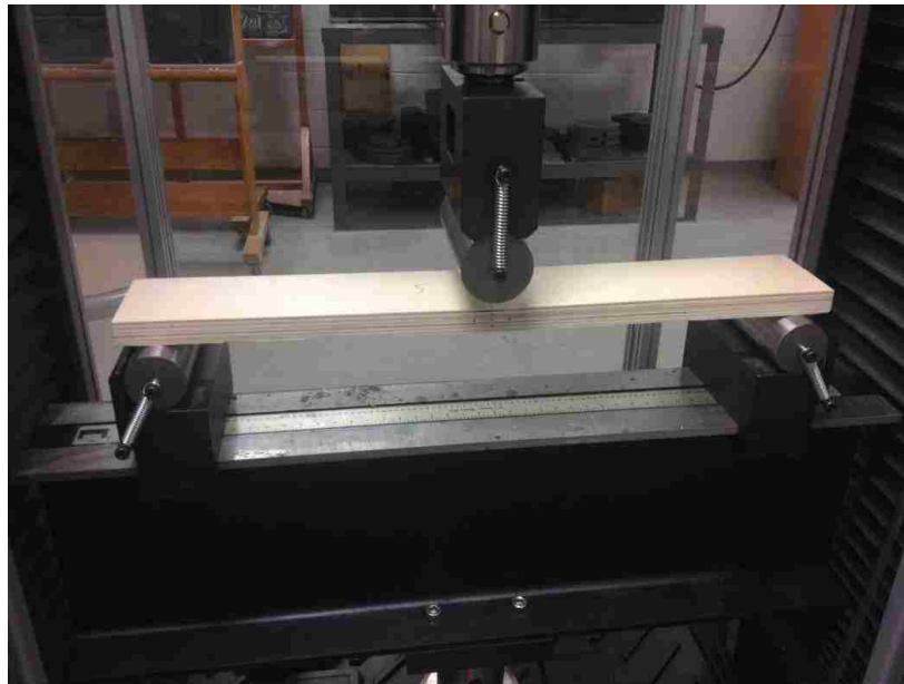
Figure 28. Test setup for three-point bending test.
