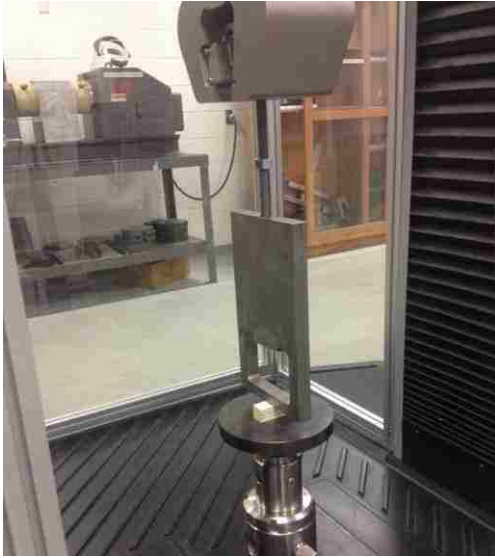
Figure 26. Test setup for the compression testing in the perpendicular direction to the wood fibre.
