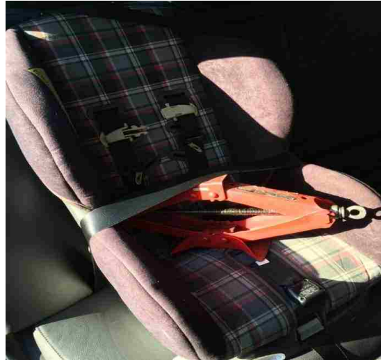
Figure 10. Simple scissor jack concept device installed on a CRS.
