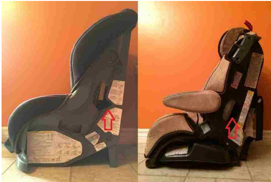
Figure 74. Difference on the lower anchor strap routing location between two CRSs (Graco Comfort Convertible on the left and Eddie Bauer Alpha Elite on the right) pointed with red arrows.
