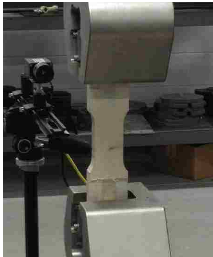
Figure 23. Tensile test setup in parallel to fibre direction with specimen placed in grip crosshead.
