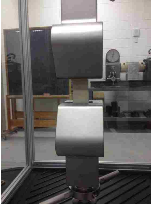
Figure 24. Tensile test setup for the perpendicular to fibre direction configuration.
