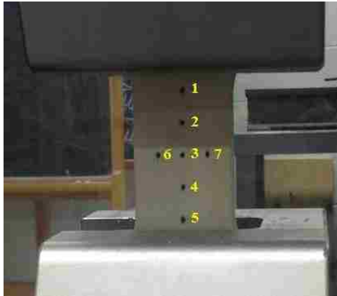
Figure 20. Hand-marked strain gauge dots (1 to 7) for video extensometer capturing.
