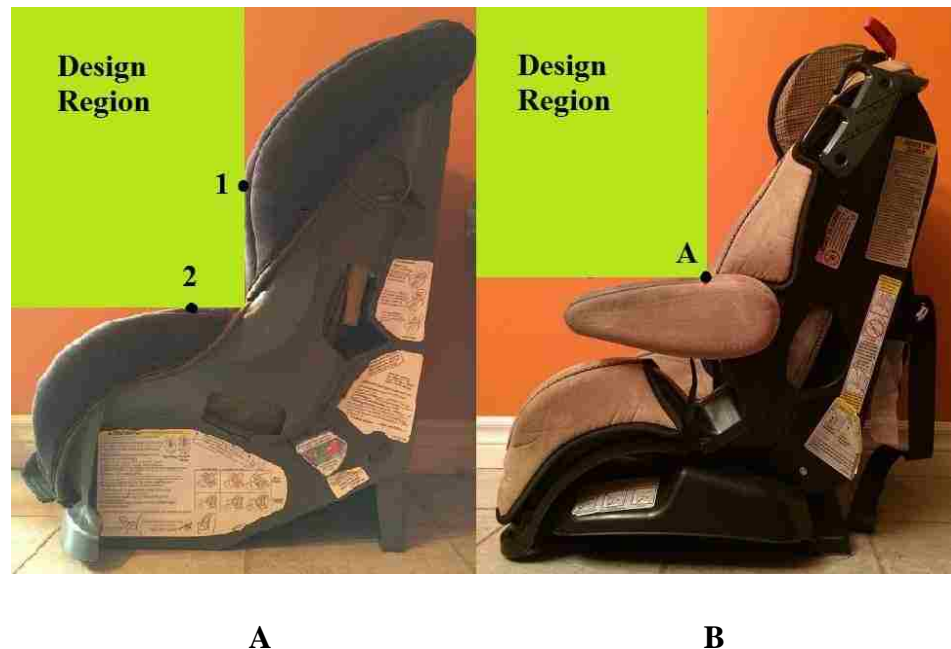
Figure 13. Sample CRSs (A: Graco Comfort Convertible with no accessory; B: Eddie Bauer Alpha Elite with armrest) to demonstrate design envelop measurement (green zone).
