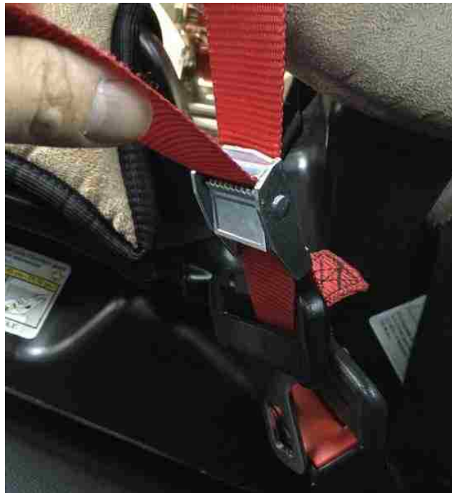
Figure 72. The steel adjustable clip applied to the ratchet webbing.
