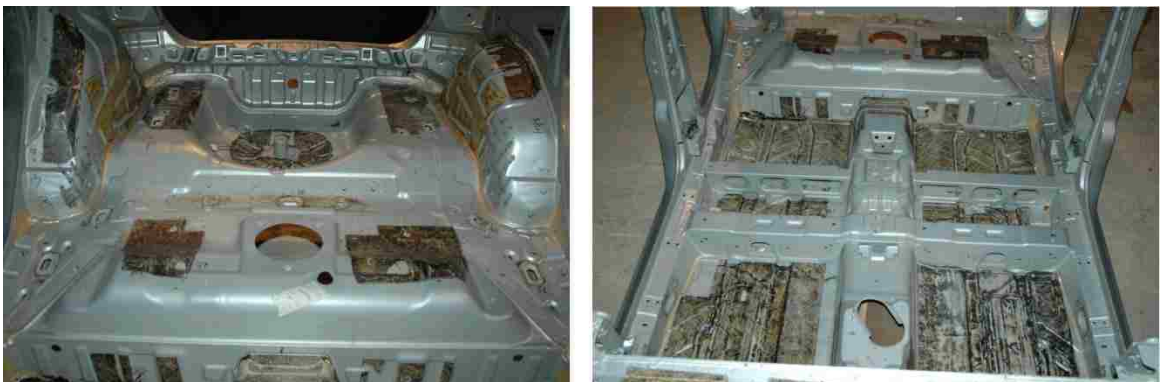
Figure 0.41: Example of damping treatments layout on a vehicle's floor.
