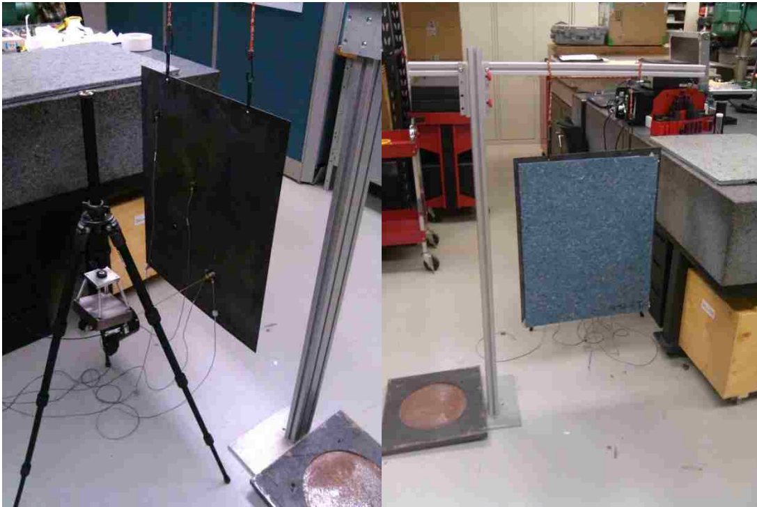
Figure 0.4: Experimental setup for the tests conducted on the steel plate.
