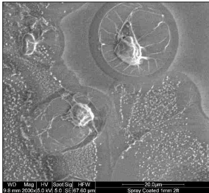
Figure 98. An ESEM image of the surface of the medium spray-coated glass with 2mm nozzle sample at 2000X magnification
