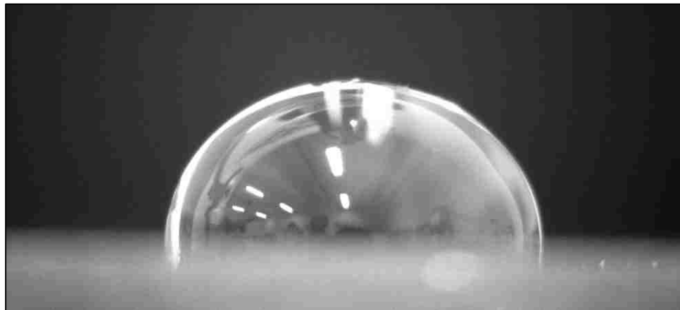
Figure 28. Profile of water droplet on polished aluminum for measuring the water contact angle
