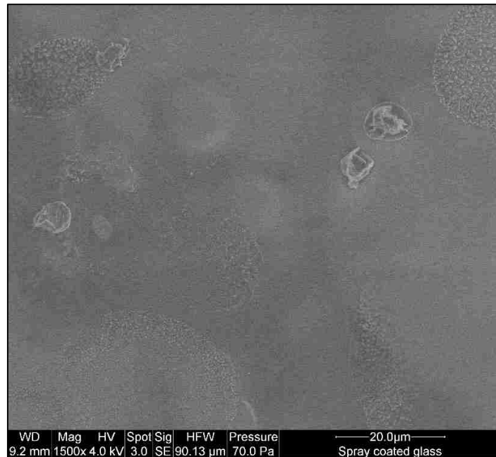
Figure 92. An ESEM image of the surface of the lightly spray-coated glass with 2mm nozzle sample at 1500X magnification
