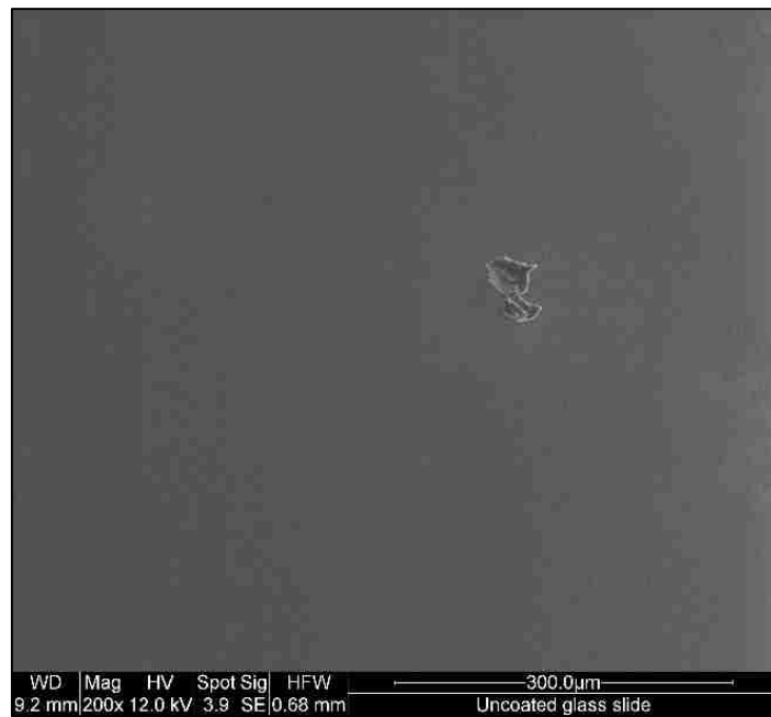
Figure 26. An ESEM image of the surface of the glass sample, a small piece of dust is visible at 200X magnification
