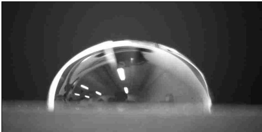
Figure 40. Profile of water droplet on polished stainless steel for measuring the water contact angle
