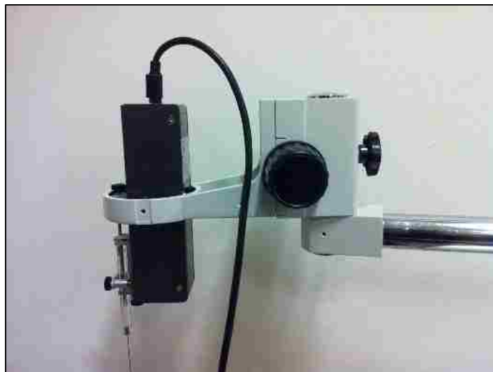
Figure 57. The rack-and-pinion mechanism allowed for repeatable precise maneuvering
