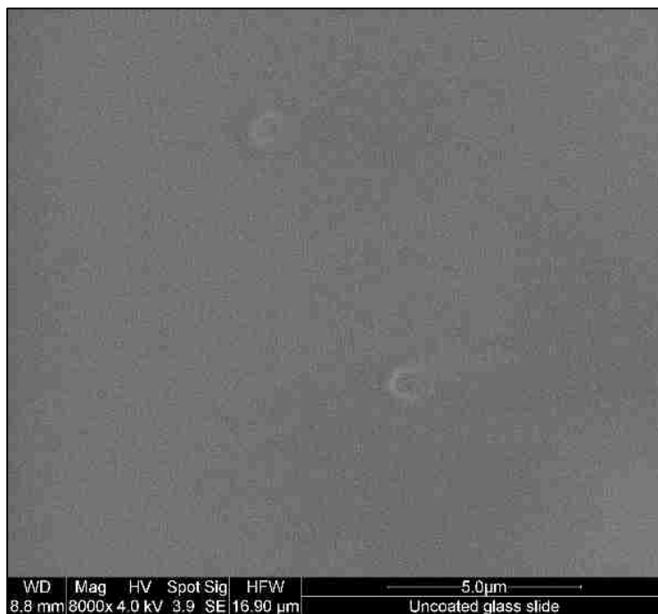
Figure 87. An ESEM image of the surface of the dip-coated glass sample, the surface exhibits small 'island' morphology at 8000X magnification
