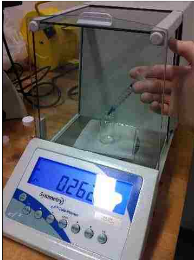
Figure 65. High accuracy balance used to precisely measure the weight of precursor chemicals
