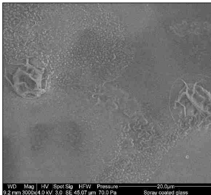
Figure 93. An ESEM image of the surface of the lightly spray-coated glass with 2mm nozzle sample at 3000X magnification
