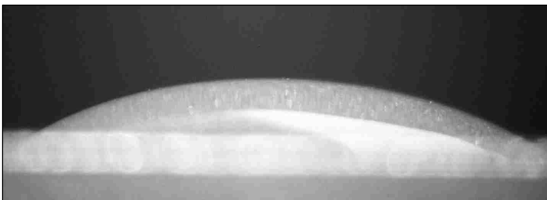
Figure 44. Profile of water droplet on moderate stainless steel for measuring the water contact angle
