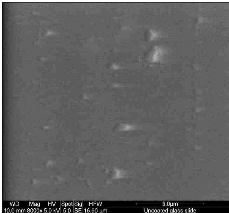
Figure 27. An ESEM image of the surface of the glass sample, at 8000X magnification small cups formations ( <1 \mu\text{m} ) are only visible features
