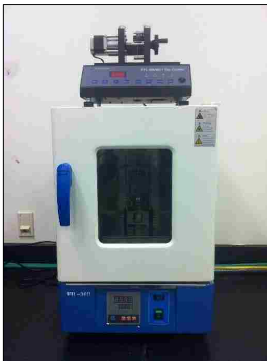
Figure 68. MTS climate controlled variable-speed dip-coater used throughout the study
