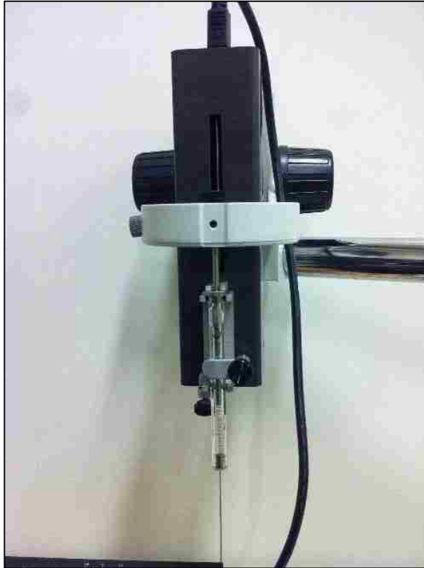
Figure 56. The computer operated driver of the syringe supported by the boom stand
