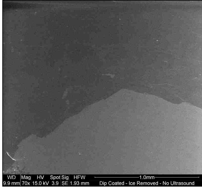
Figure 152. An ESEM image of the surface of the dip-coated glass sample after ice shedding event at 70X magnification
