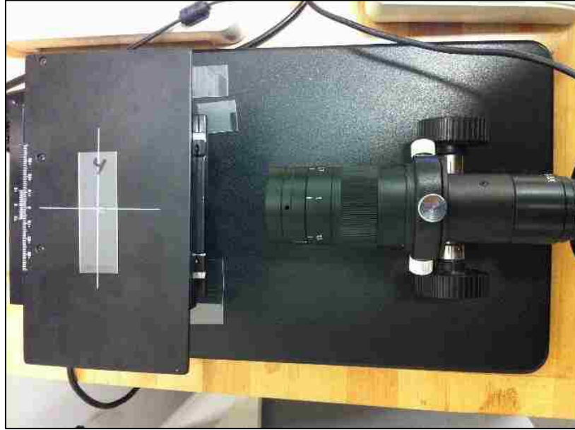
Figure 54. The horizontal microscope stage used in the construction of the goniometer
