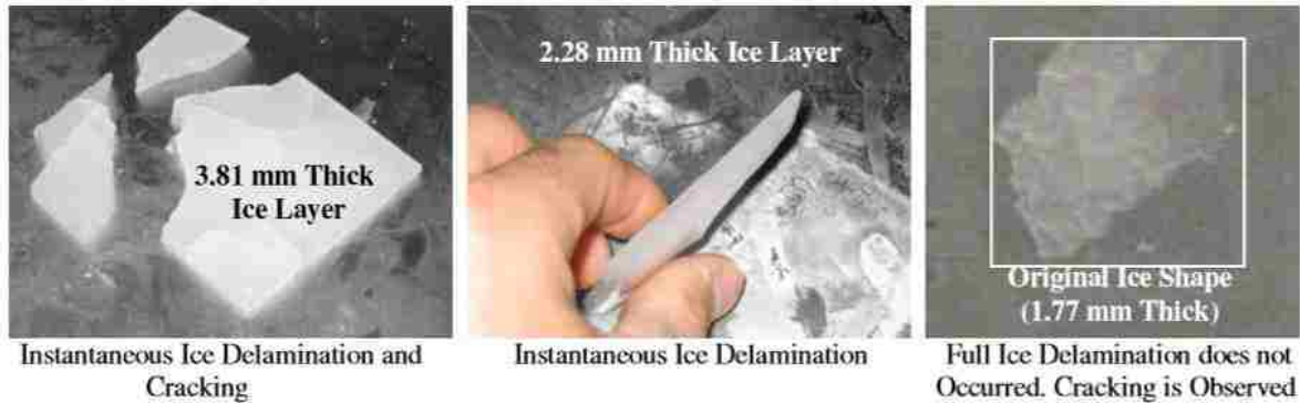
Figure 11. Stresses \sigma_{zx} is zero at the elements free traction surface, but promotes delamination between a host structure and accreted ice layer. The ice layer will also undergo \sigma_{xy} stresses through its thickness (stress responsible for ice cracking) (25)
