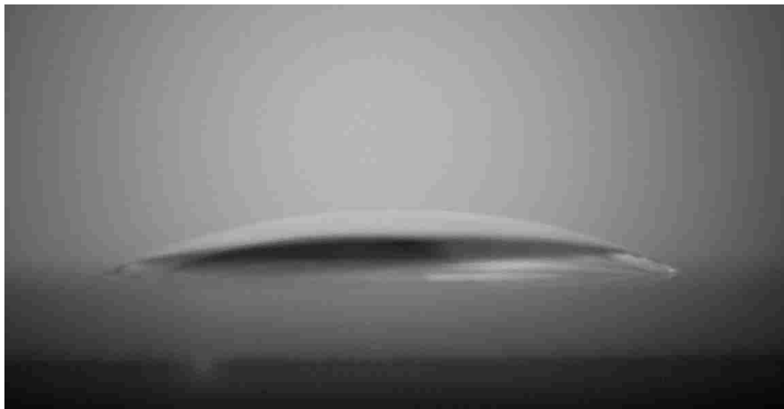
Figure 21. Profile of water droplet on glass for measuring the water contact angle
