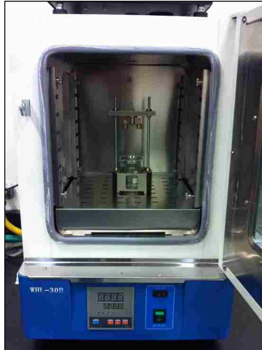
Figure 69. A view inside the MTS climate controlled variable-speed dip-coater showing the retractable dipping stage
