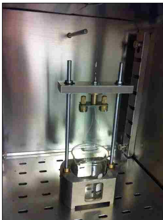
Figure 72. A close-up view inside the dip-coater showing the stage lowering a glass slide into the solution beaker
