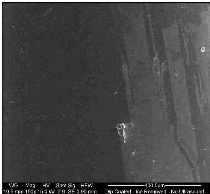
Figure 153. An ESEM image of the surface of the dip-coated glass sample after ice shedding event at 150X magnification
