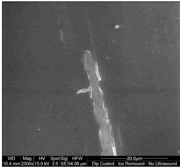
Figure 155. An ESEM image of the surface of the dip-coated glass sample after ice shedding event at 2500X magnification
