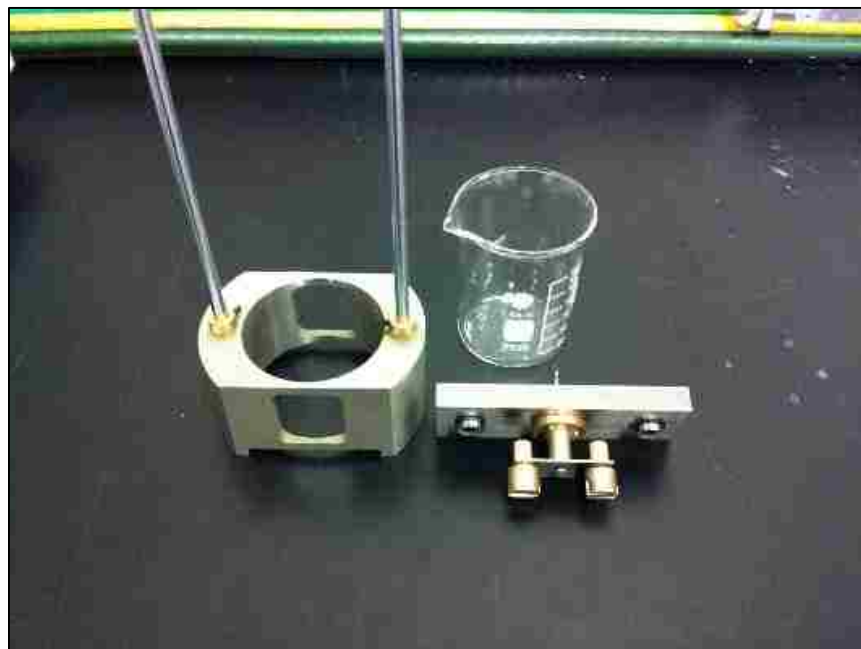
Figure 70. A close-up image of the coating solution beaker, the beaker holder with guide rails, and the mounting stage for fastening test slides
