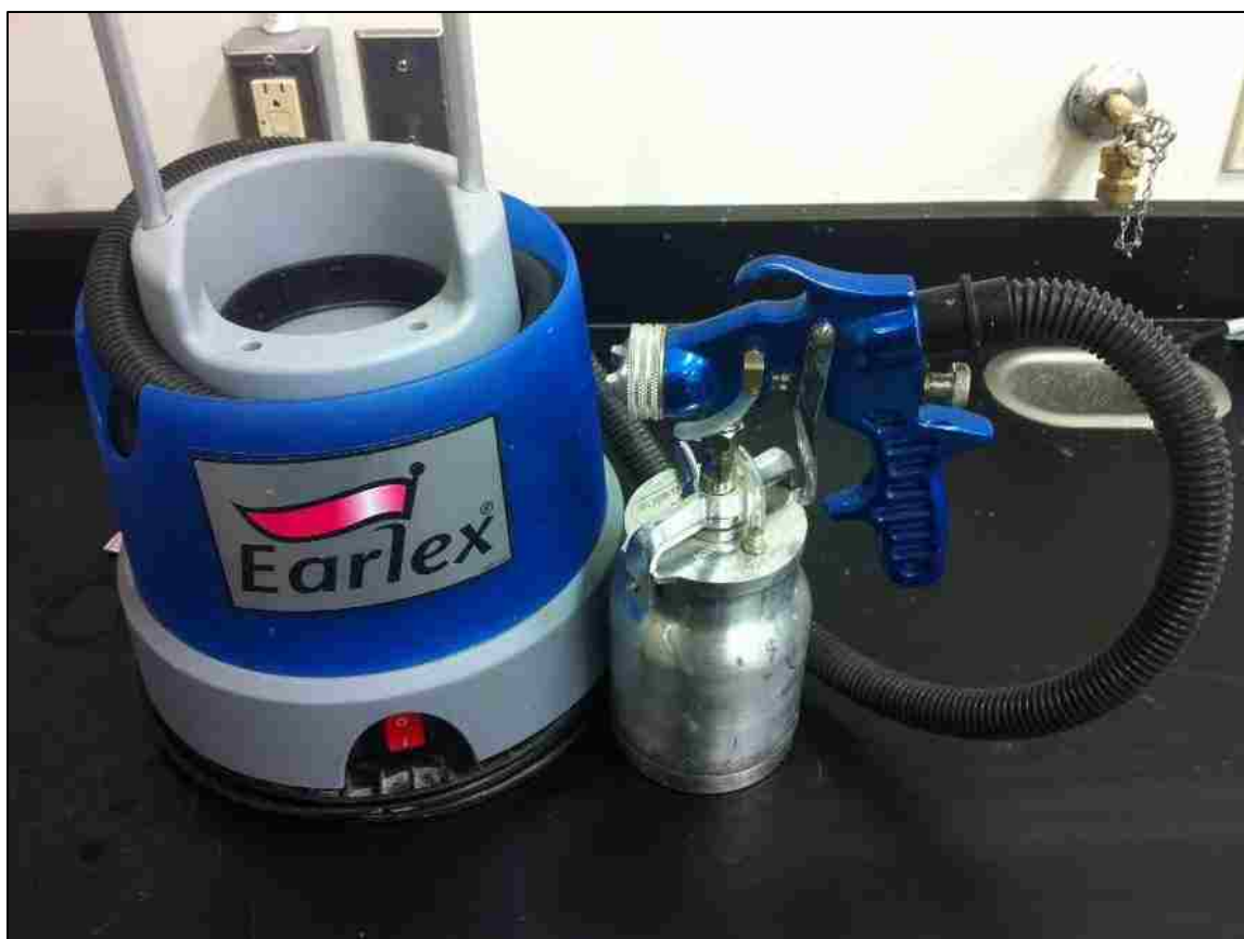
Figure 73. The Earlex spray-coater used to deposit the rough sprayed coatings
