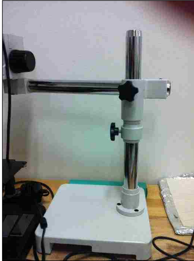
Figure 58. The boom stand could be adjusted and fixed in any convenient location
