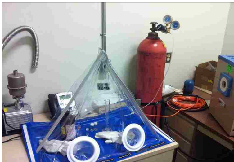
Figure 66. Chemical precursors were mixed in glove bag under argon atmosphere
