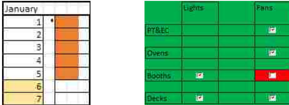
Figure 3.2 – Detail of the calendar module and part of the shutdown selection panel
