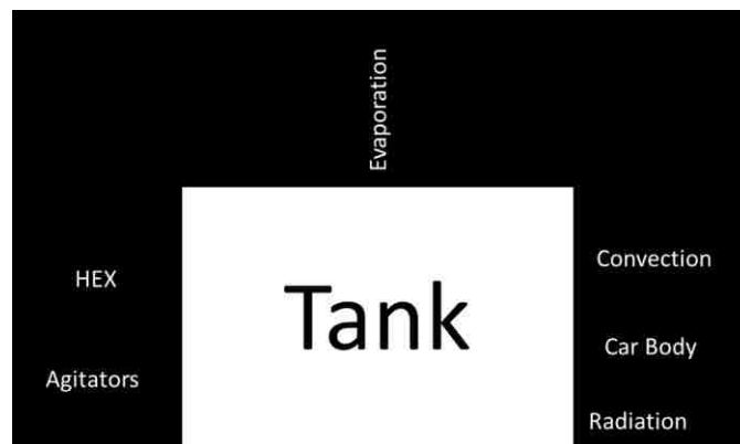
Figure 3.5 – Dip tanks heat transfer schematics
