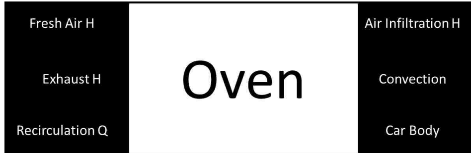
Figure 3.9 – Oven heat loss diagram
