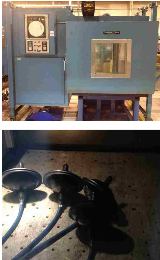
Figure 3.5 Pressure cycle fatigue testing machine and test set-up
