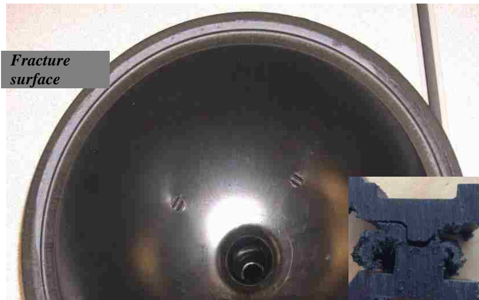
Figure 3.12 Fractured sample underwent a burst test
