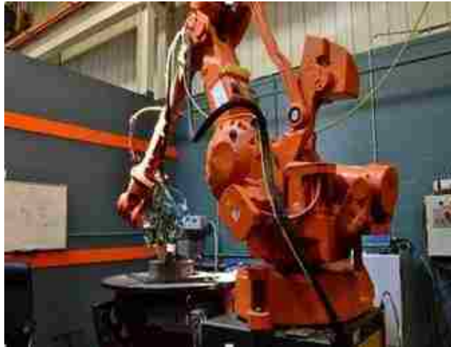
Figure 19. Laser Cladding work cell utilized for this research [Courtesy to industrial partner]
