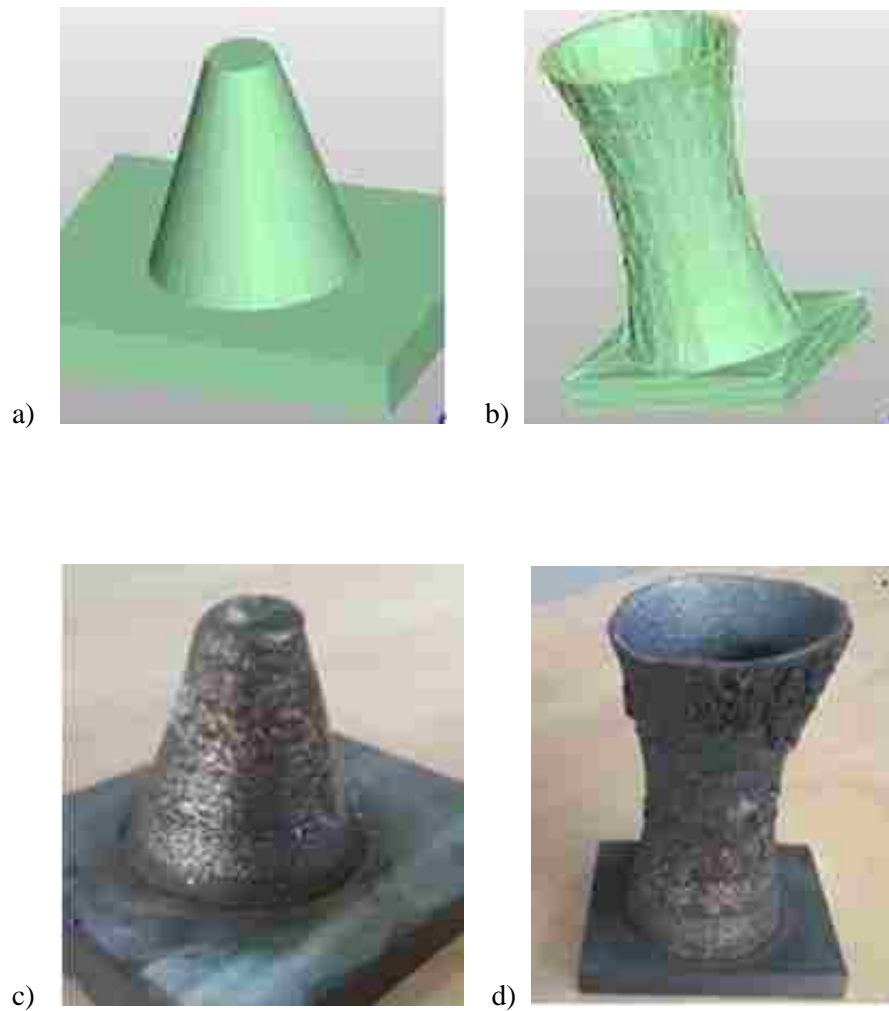
Figure 41. Models made using laser cladding method a) b) CAD models c) Hollow cone model d) Parabolic shape model
