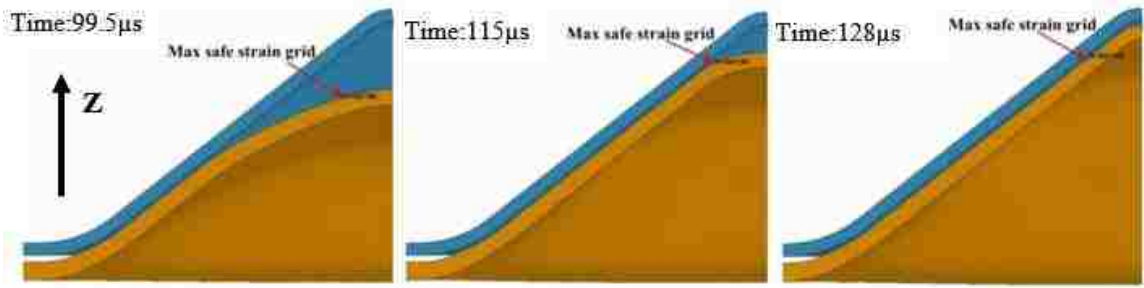
Figure 5.22. Position of the grid that reaches the maximum safe strain at distinct moments during the deformation of the V-shaped specimen
