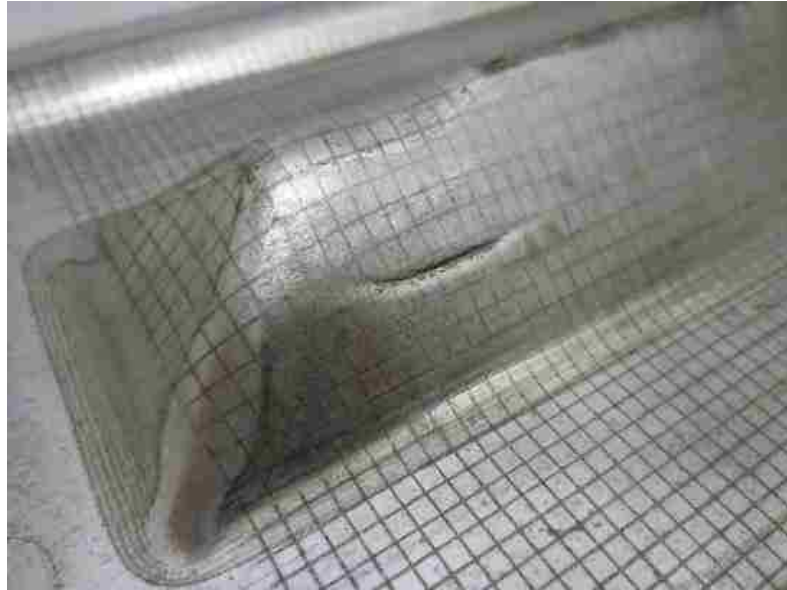
Figure 5.4. Crack in a 1.5 mm DP600 specimen formed into the 38° V-shaped die using a 14 kV pulse
