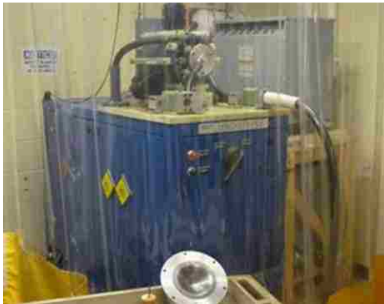
Figure 3.5. Magnepress power supply module
