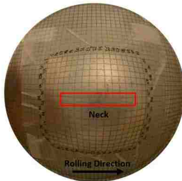
Figure 5.41. EHFF specimen formed in balanced biaxial tension using 13.6kV
