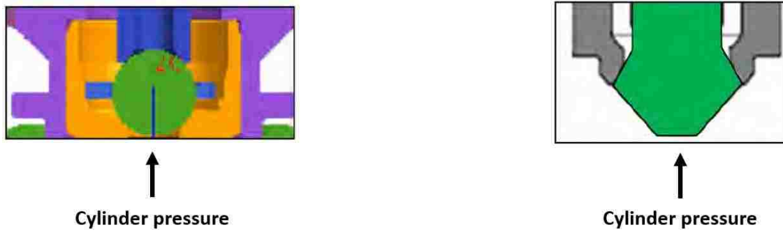
Figure 2.18: Inward opening and outward opening valve scheme for a DI injector [4]
