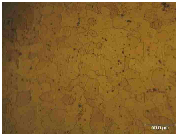
Figure 5.1: Optical microscope image of the aluminum alloy 7046, solutionized at 480 °C for 2 hours. The microstructure was revealed with immersion in the Kellers etchant for 30 seconds.
