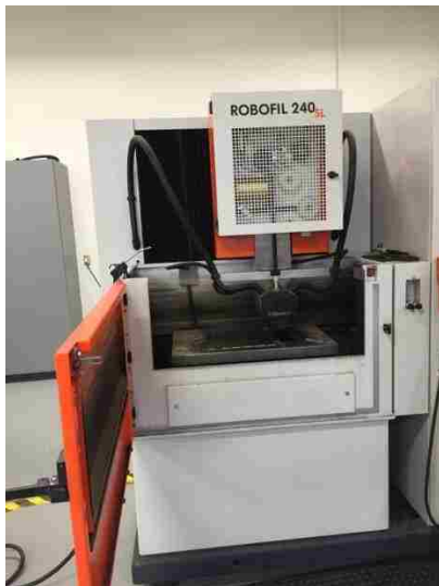
Figure 4.3 On the left, the EDM machine used for cutting the specimens. On the right, the aluminum sheet placed in the machine before being cut.
