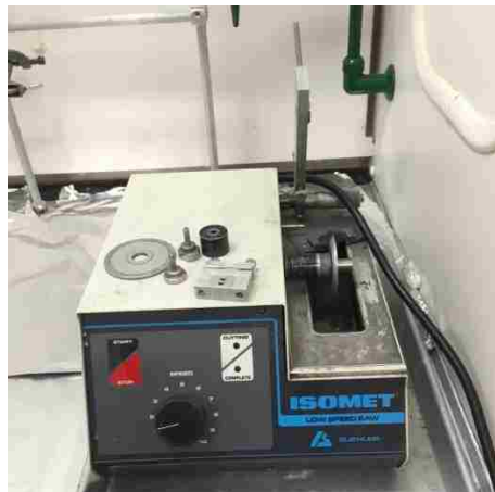
Figure 4.6: Cutting machine used for the preparation of the samples for the microstructural analysis
