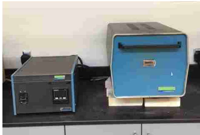
Figure 4.5: Furnace used for the solutionizing and ageing phases
