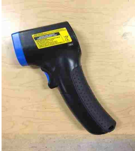
Figure 4.16: On the left, a non-contact infrared thermometer. On the right, a thermocouple.
