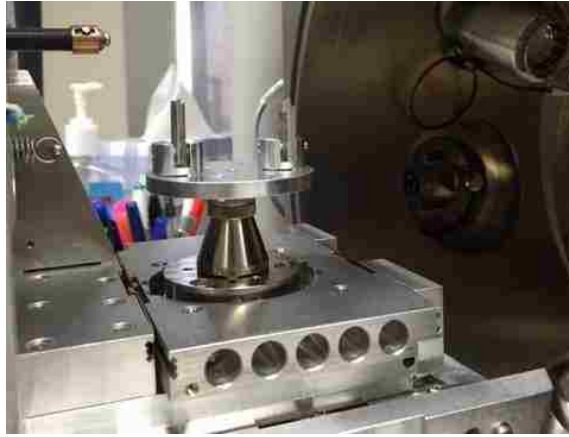
Figure 4.17: samples positioned for the fracture surface analysis with the SEM
