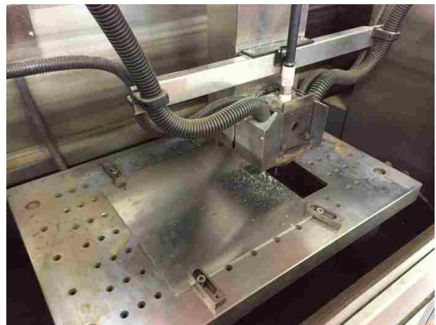
Figure 4.3 On the left, the EDM machine used for cutting the specimens. On the right, the aluminum sheet placed in the machine before being cut.
