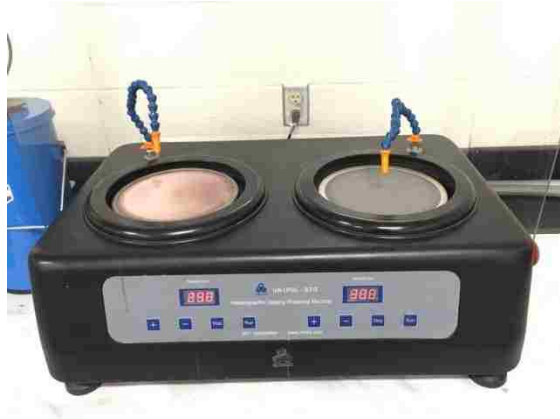
Figure 4.7: Polishing machine used for grinding and polishing
