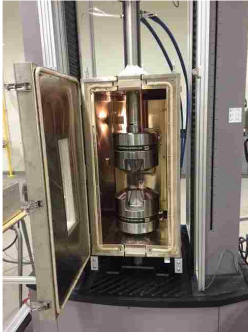
Figure 4.15 Internal part of the environmental chamber, used for the tensile tests at high temperature
