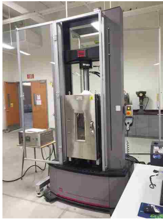
Figure 4.14: Tensile machine with the environmental chamber
