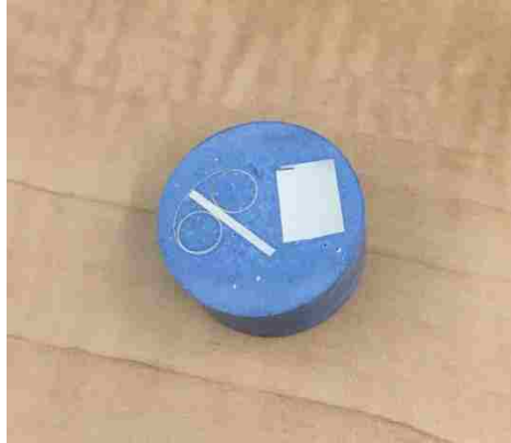
Figure 4.8: Mounted sample ready for microstructural observation
