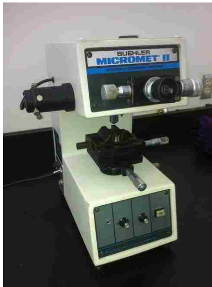
Figure 4.11: Buehler Micromet II microhardness testing machine used for the tests
