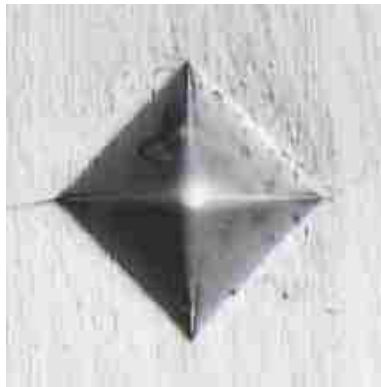
Figure 4.10: Optical micrograph of a Vickers indentation [58]
