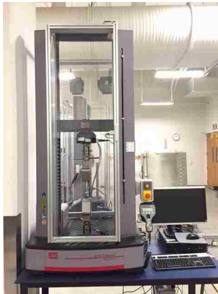
Figure 4.12: Tensile machine for the tests at room temperature
