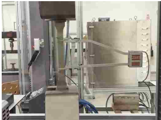
Figure 4.13: Extensometer in position during the tensile test
