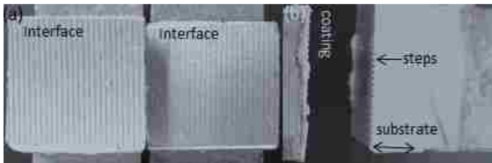
Figure 4-33 Stereo micrographs taken from the failure surfaces of the PTWA-B coating. (a) Top view of the failed surface showing the keyhole pattern made on aluminum prior to the deposition of the PTWA-B coating, (b) side view of the failed surface showing the detachment of the PTWA-B coating from the substrate at the coating/substrate interface; (c) a high magnification view of the failed surface shown in “b” illustrating the detachment of the coating at the aluminum substrate interface and the keyhole pattern made on the Al surface prior to the coating deposition.
