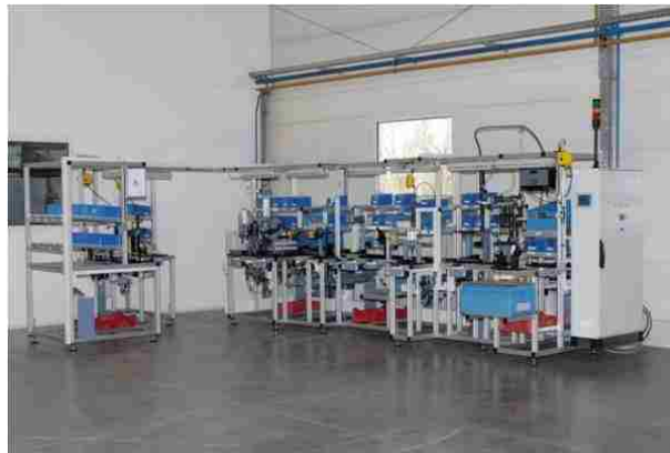
Figure 3.9 Automated Valve assembly line (Delta-Tech).
