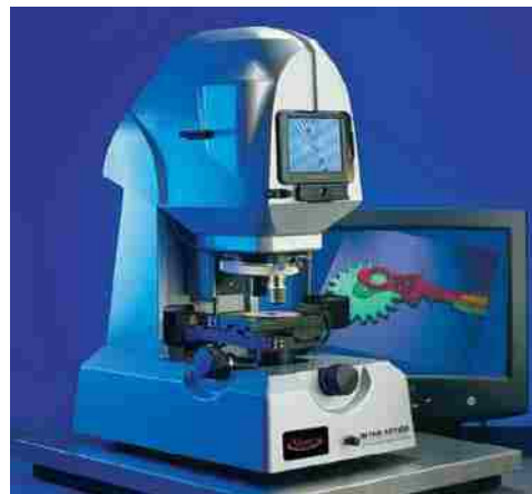
Figure 3.3 WYKO optical profiling microscopy including the full Wyko Vision® analytical software package
