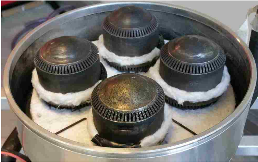
Figure 3-5 Photograph of internal heat exchanger
