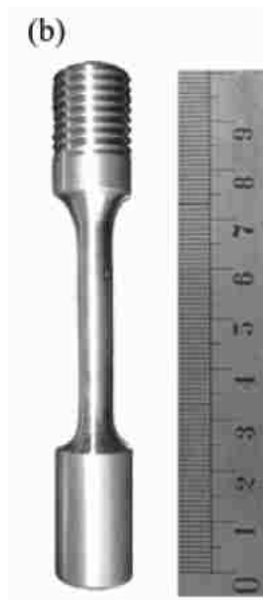
Figure 2.13 [19] Ultrasonic-vibration apparatus (a) and AZ31 sample for tensile testing (b).
